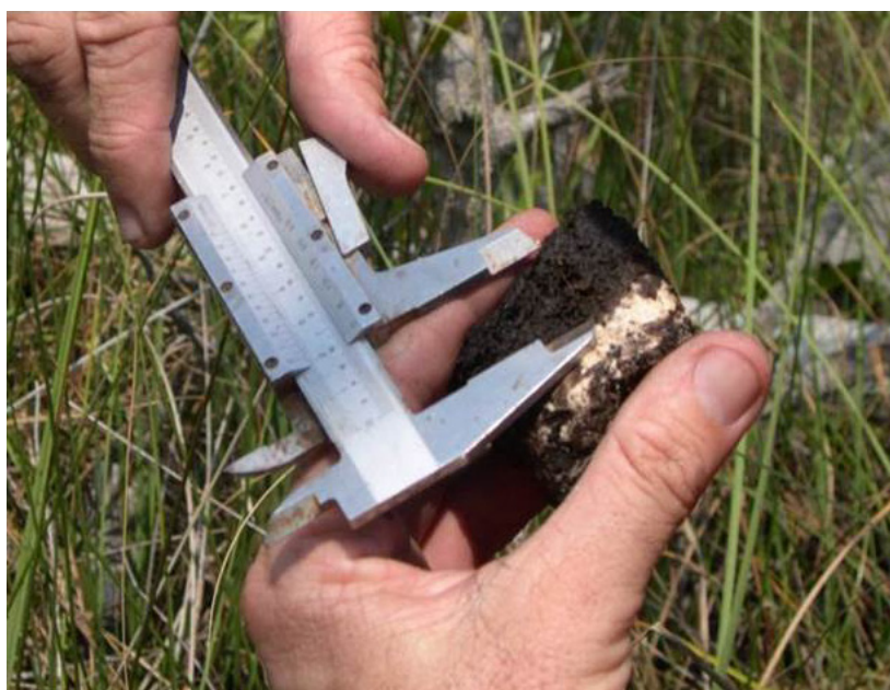
FIGURE 5-9 Measurement of soil accretion using the marker horizon method in Everglades National Park. In this method, researchers place a layer of feldspar clay (visible as a white layer) on the surface of the marsh and later return to measure the soil that has accumulated. The marker horizon method is often used in conjunction with a sediment elevation table (SET) to measure total soil accretion or erosion.
