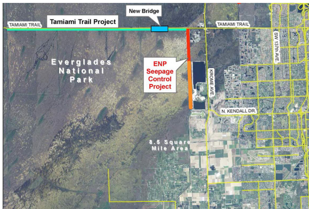
FIGURE 4-20 Position of the 2-mile-long, 35-foot-deep seepage barrier (shown in red), west of the L-31N Canal. The orange line represents a possible 3-mile extension of the project.
