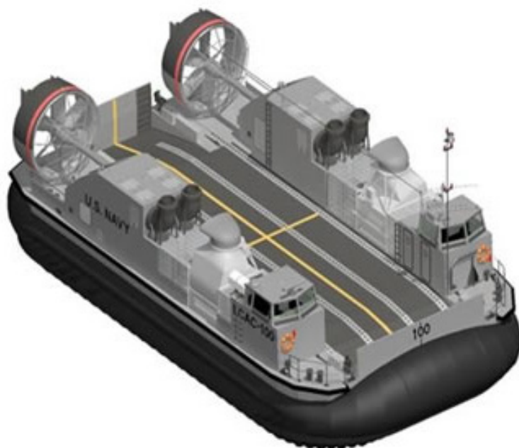
FIGURE 4-9 Artist's concept of an SSC. SOURCE: U.S. Navy, "PEO Ships Ship-to-Shore Connector (SSC)," http://www.navsea.navy.mil/teamships/PEOS_SSC/SSC_Images.aspx .
