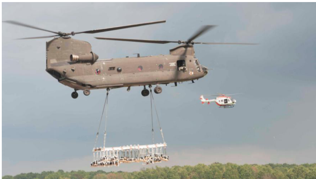
FIGURE 4-19 Helicopter sling for delivering cargo by JPADS, during testing. SOURCE: Keith Bowman and Daniel Schreiter, Precision Airdrop Program Office, AFRL, “AFRL Precision AirDrop (PAD) Update,” presentation to the committee on February 5, 2014.
