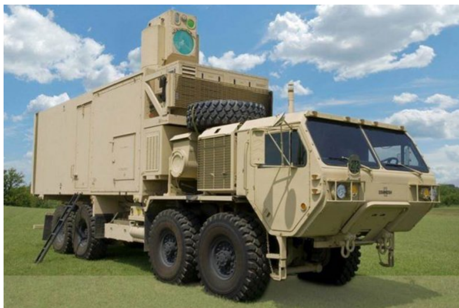
FIGURE 3-2 The High-Energy Laser–Mobile Demonstrator (HEL-MD). The beam director is on top. SOURCE: Army vehicle-mounted laser successfully demonstrated against multiple targets, www.army.mil/article/116740/Army_vehicle_mounted_laser_successfully_demonstrated_against_multiple_targets/ .
