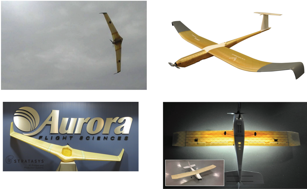
FIGURE 1.6 Examples of small aircraft produced partially or entirely with additively manufactured parts by Aurora Flight Sciences. The increasing sophistication of machines produced with additive manufacturing technology is relevant to the in-space production of parts and even entire small spacecraft. SOURCE: Courtesy of Aurora Flight Sciences.
