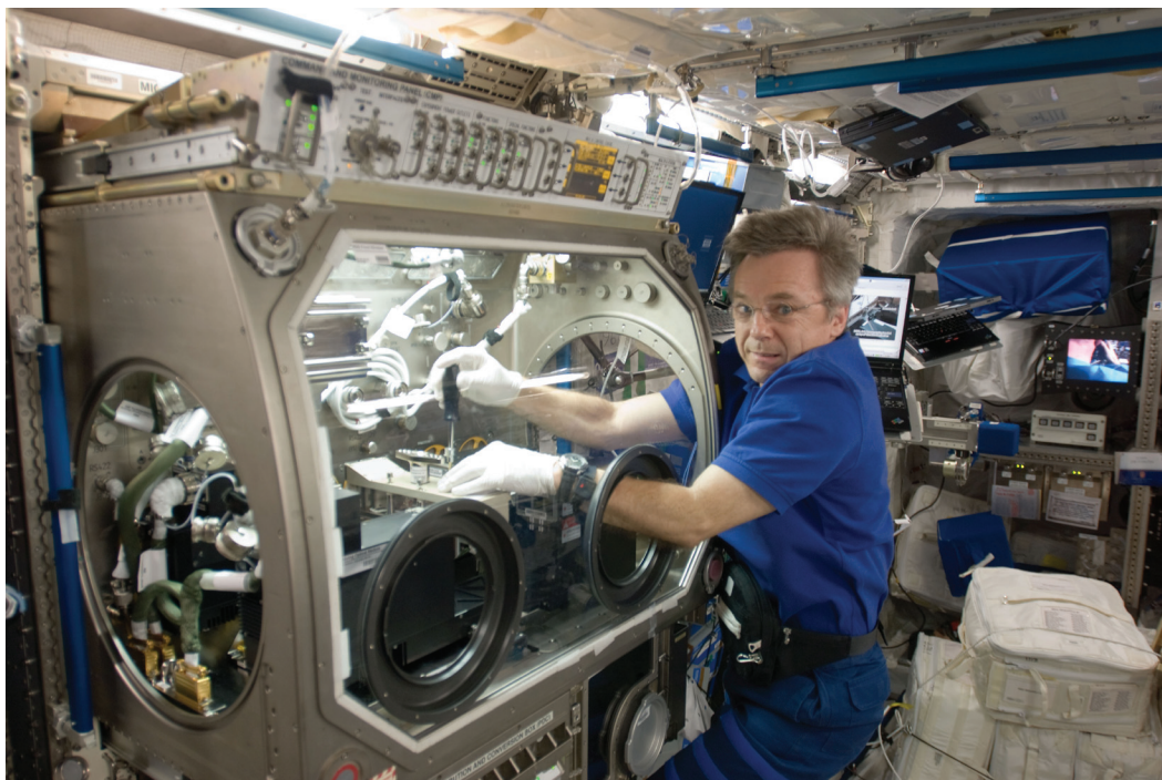
FIGURE 3.4 Microgravity glovebox on the International Space Station (ISS). The ISS has equipment that can be used for additive manufacturing experiments. Any such experiments will naturally have to compete with other research priorities. SOURCE: Courtesy of NASA.
