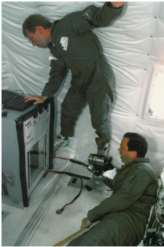
FIGURE 1.14 A 1999 test aboard a KC-135 “Vomit Comet” of an original fused-deposition modeling device. These flight tests were conducted by Cooper and Griffin. This early work, sponsored by NASA’s Marshall Space Flight Center, was the forerunner to the upcoming International Space Station experiments. SOURCE: Courtesy of NASA.
