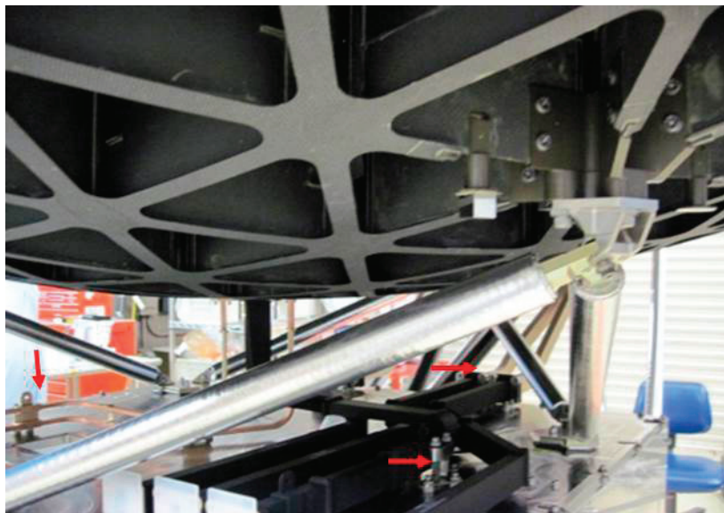
FIGURE 1.5 Additively manufactured waveguide brackets (shown by red arrows) installed on the Jupiter Juno spacecraft during assembly. SOURCE: Courtesy of Lockheed Martin.
