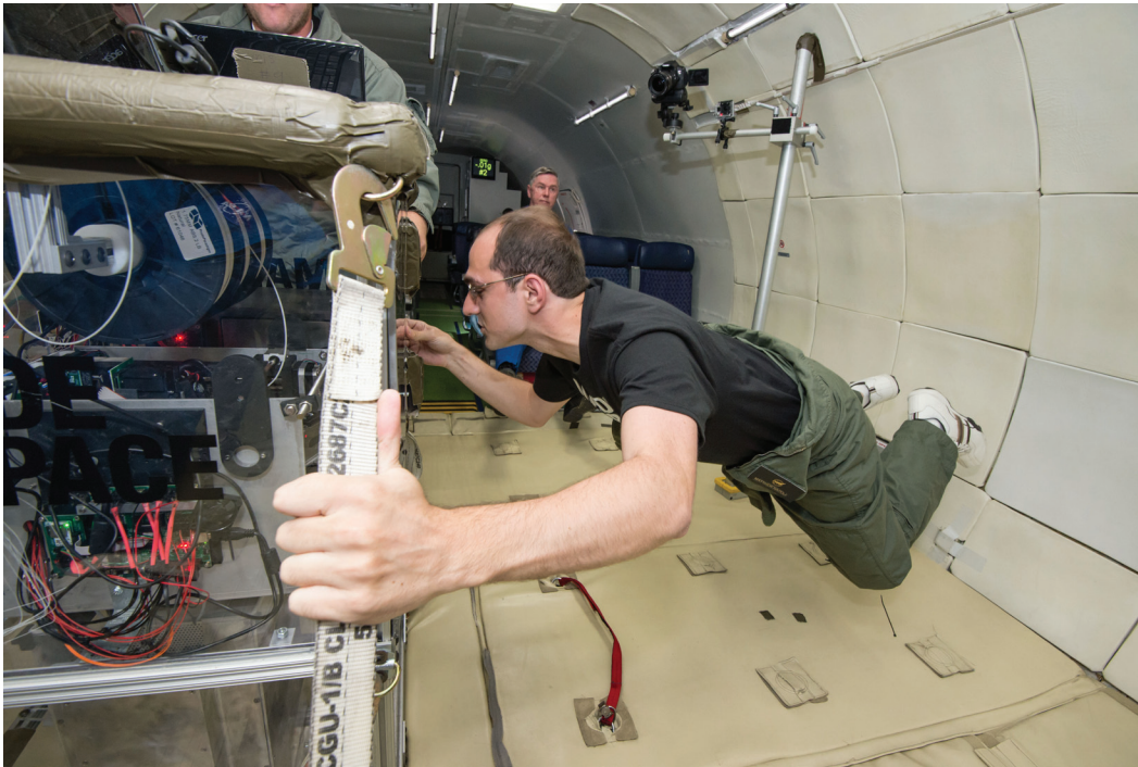
FIGURE 1.15 3D printer developed by Made In Space, Inc., for testing aboard the International Space Station undergoing microgravity testing aboard a parabolic aircraft in 2013. SOURCE: Courtesy of Made In Space, Inc.
