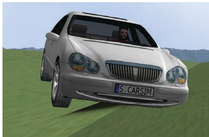
Figure 5-16. Bumper ground penetration.
