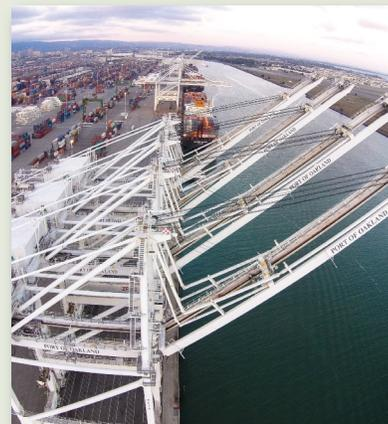
COVER: In 2016, a major expansion of the Panama Canal will facilitate passage of vessels up to 15,000 TEUs and with drafts of 50 feet. The large vessels will require super-post-Panamax crane and draft equipment, shown here at the Port of Oakland. (Photo: Eddie Codel, Port of Oakland)
