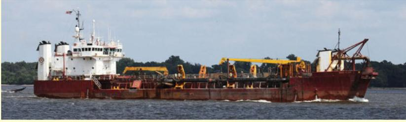
A Great Lakes Dredge and Dock Company hopper dredge works to remove approximately 400,000 cubic yards of material from the Delaware River near Philadelphia, Pennsylvania. Larger vessel sizes have required many infrastructure upgrades at ports and inland waterways.
