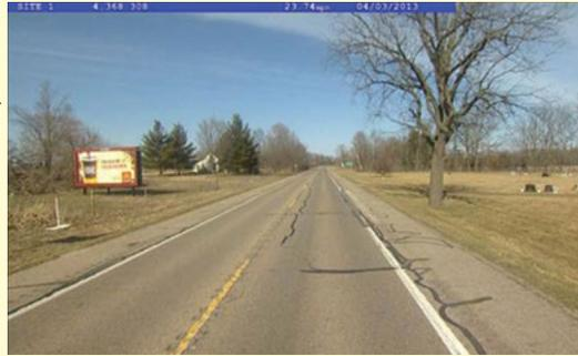
A Michigan DOT pilot project tested remote sensing technologies to monitor highway assets. With asset extraction software, users can zoom in on multiple points in a single image.
