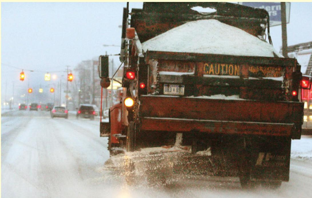
A salt truck applies deicing material before a storm in Wayne County, Michigan. Strict stormwater regulations have caused state DOTs to examine deicing applications that use sodium chloride.
