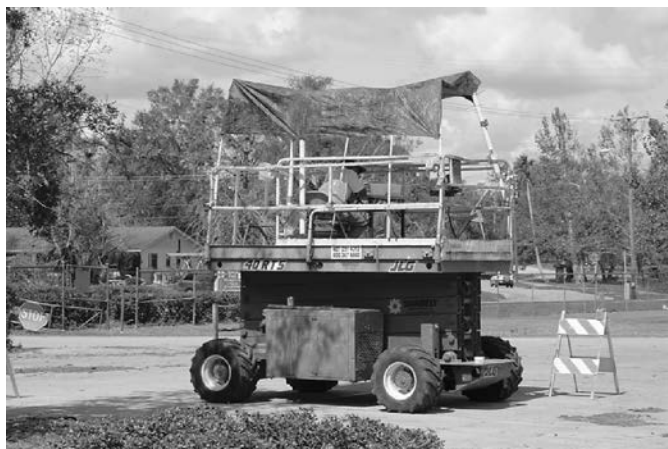
Figure 10.5. Acceptable tower monitoring station. Scissor lift with terrain tires. (Source: FEMA)
