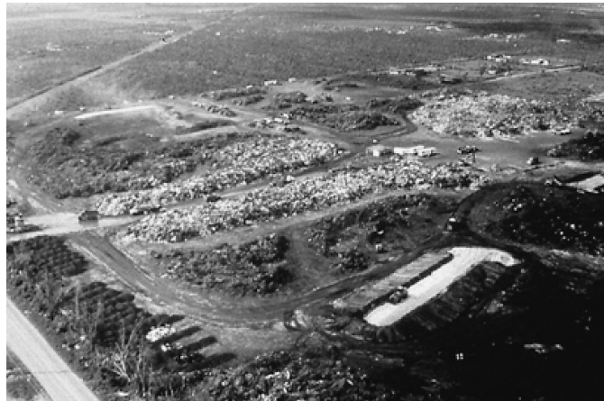
Figure 9.3. Proper site layout. The size of this DMS was approximately 100 acres and shows separate areas for burning, grinding, and recycling. (Source: FEMA)
