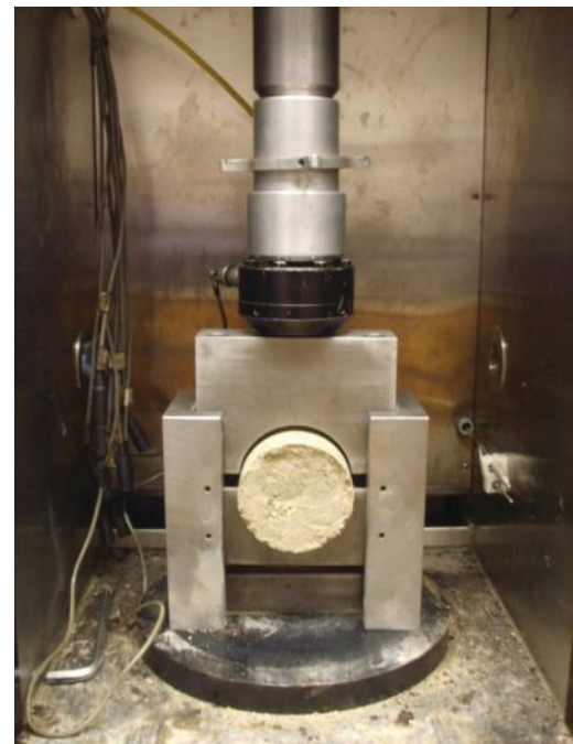
Figure 3-20. Coefficient of friction test setup.
