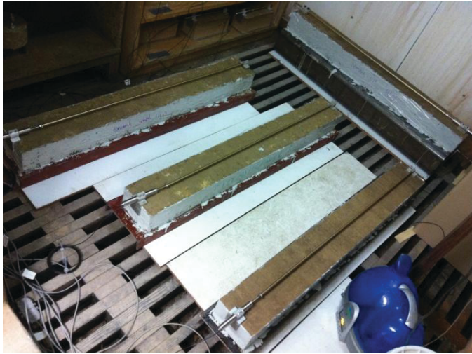
Figure 3-18. Restrained shrinkage test setup with sides sealed.
