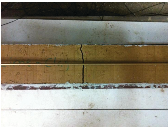
Figure 3-19. Transverse crack in clay-lime specimen (view from top).
