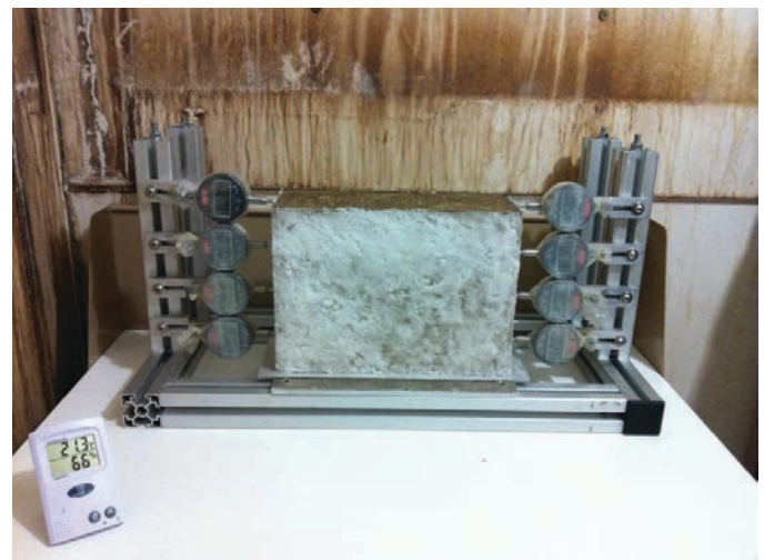
Figure 3-16. Free-drying shrinkage with moisture gradient test setup.
