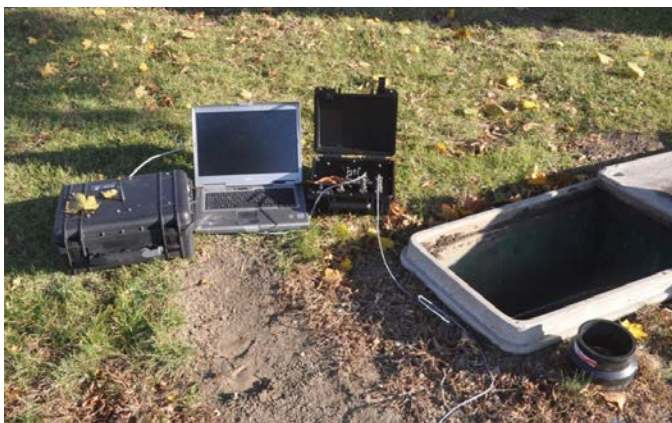
Figure 4.5. Active injection equipment being tested at Manteno.
