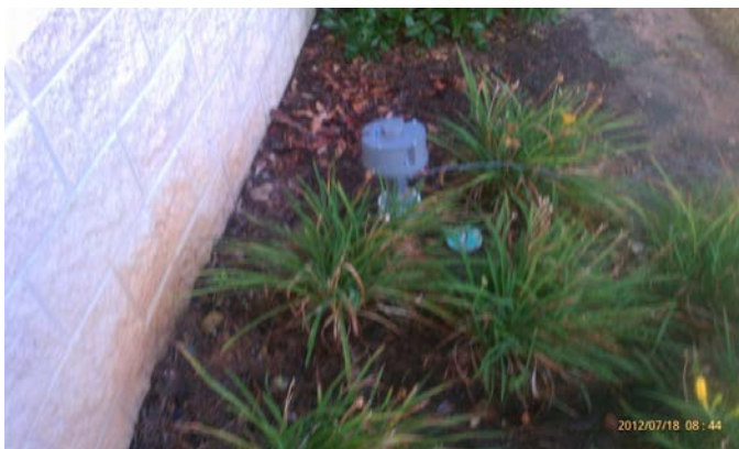
Figure 4.9. Speaker on clean out near 1130 Talbotton.
