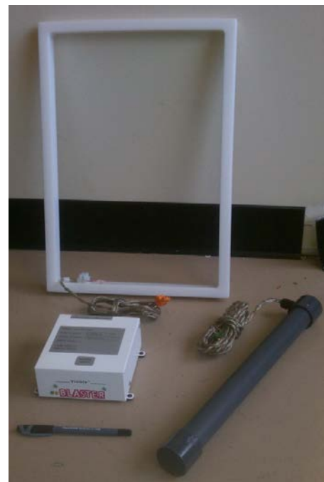
Figure 4.22. Base station tag reader with two alternative antennas.
