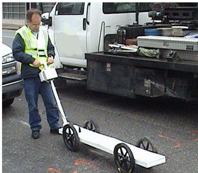
Figure 3.6. GTI metallic joint locator.
