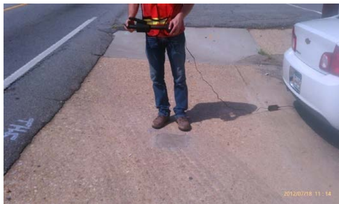
Figure 4.23. Using V-Rod to locate two tags buried near 2039 Warm Springs Road.
