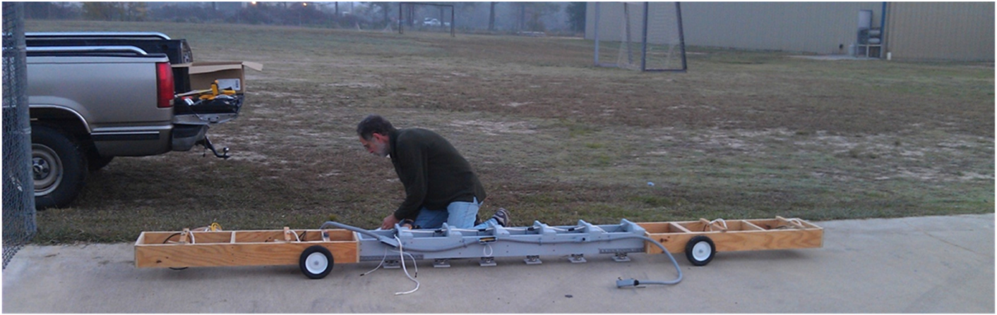
Figure 4.1. Seismic reflection initial prototype.
