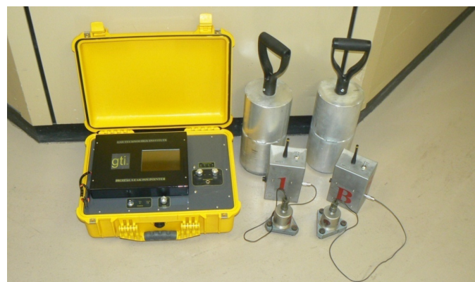
Figure 3.4. GTI digital acoustic leak detector.
