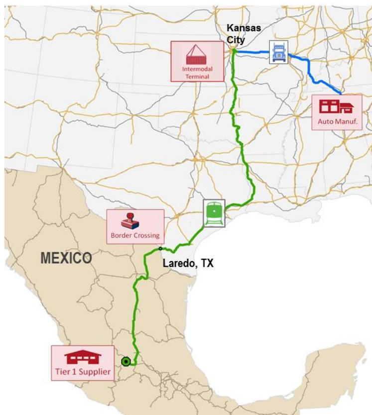
**FIGURE 18 General Motors automotive supply chain example: Mexico to Spring Hill by rail and truck. (Source: Prepared by Cambridge Systematics, Inc., and Parsons Brinckerhoff for the I-95 Coalition.)**
