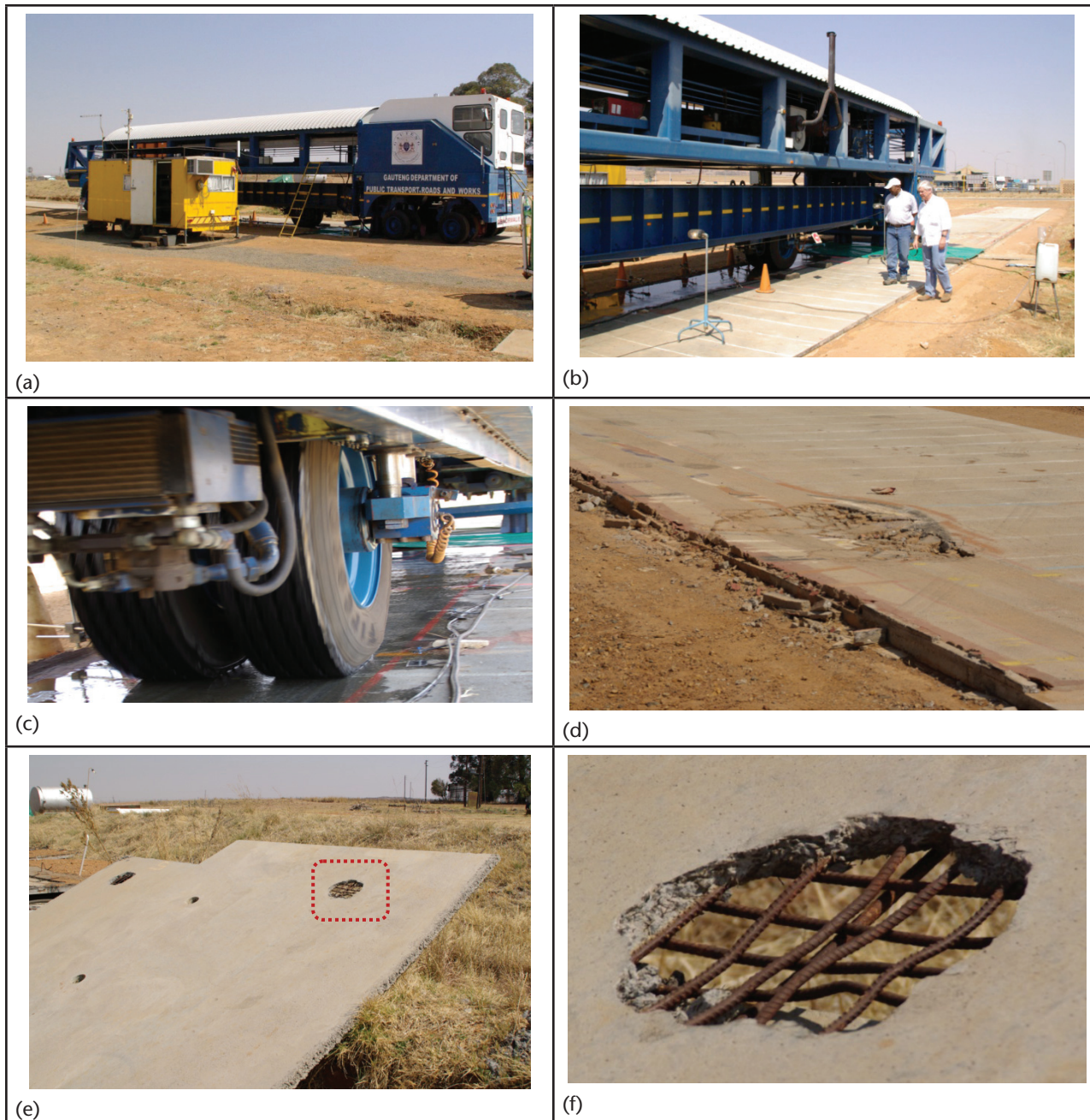
Figure 6.1. Thin CRCP being tested via the heavy vehicle simulator in South Africa. (a) Testing of thin CRCP near Heidelberg, South Africa. (b) HVS testing of 50-mm thin CRCP. (c) Testing includes substantial instrumentation for in situ measurements. (d) HVS testing typically continues until a failure condition is reached. (e) Previously tested section illustrating reinforcing. (f) Close-up of reinforcing. Photos: Joe Mahoney.
