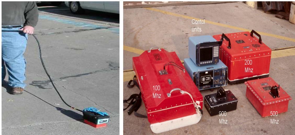
Figure 1.16. Ground-coupled systems: 1.5 GHz (left); lower-frequency antennas with control unit (right).
