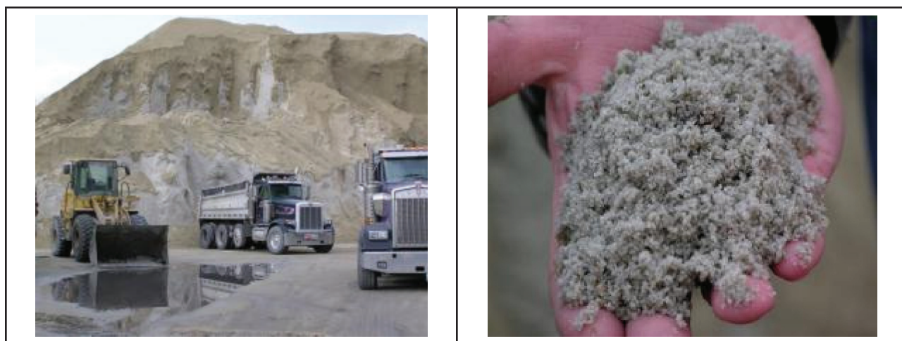
Figure 3.13. Preprocessed blast furnace slag.
