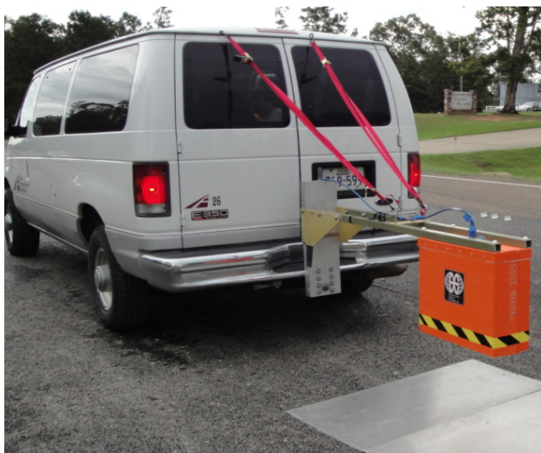
Figure 1.15. Air-coupled GPR systems for highways.
