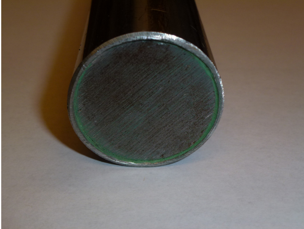
Figure 3.20. Stainless steel dowel bar. Photo: Joe Mahoney.
