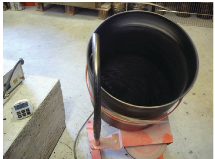
Figure 1.12. Bucket mixer used for mix verifications.
