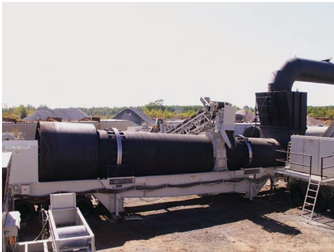
Figure 1.18. Portable asphalt plant used for Iron Mountain, Michigan, project (19).
