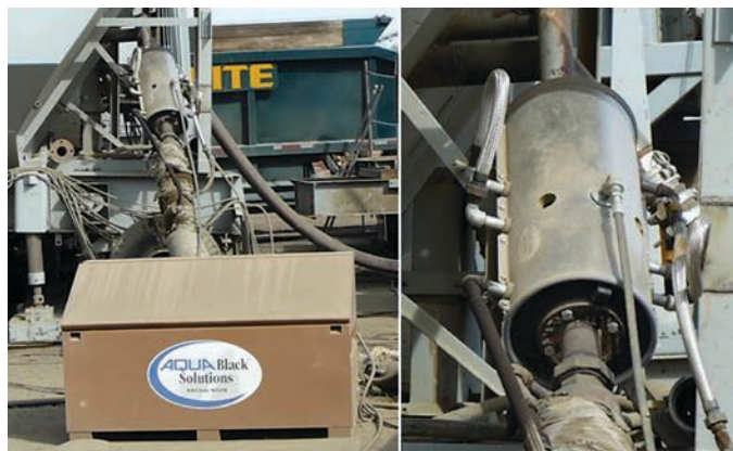
Figure 1.40. AQUABlack WMA system used in Walla Walla, Washington.
