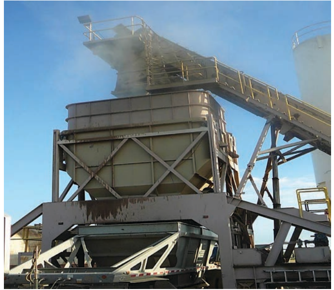
Figure 1.74. Portable parallel-flow drum plant in Baker, Montana.
