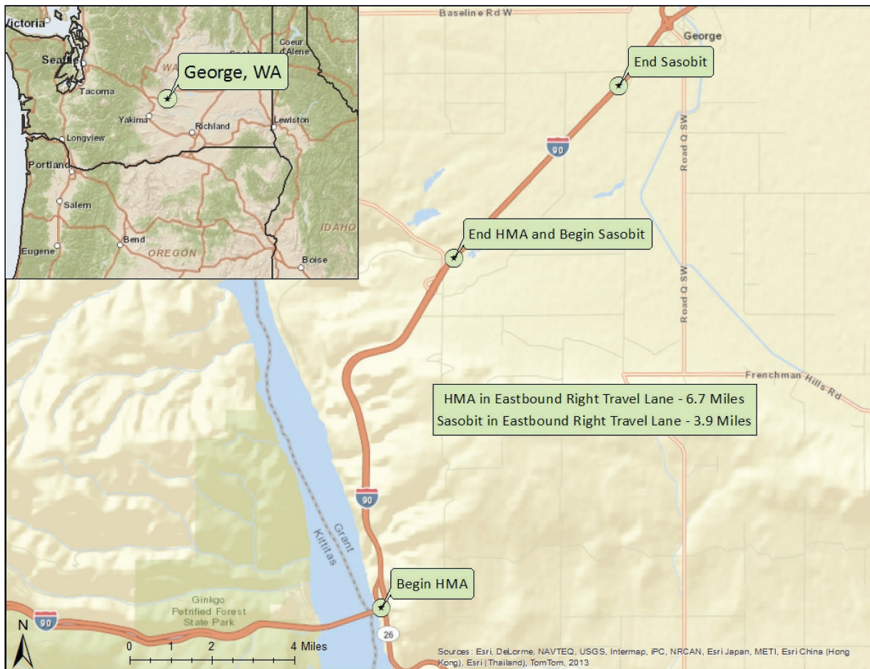
Figure 1.35. Locations of test sections in George, Washington.
