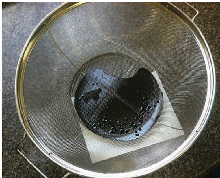
Figure 1.142. Hydrofoamer (left), polymer strained out of Florida PG 76-22 binder (right).
