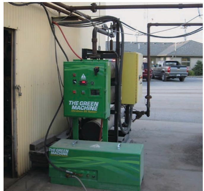
Figure 1.82. Ultrafoam GX2 foaming system used in Munster, Indiana.
