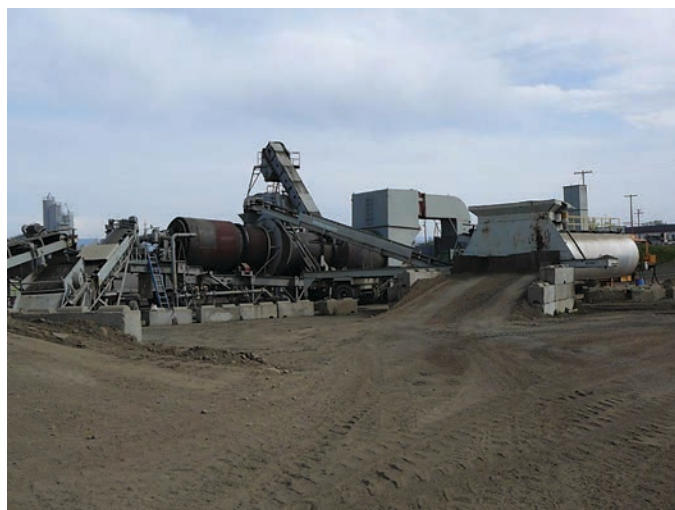
Figure 1.41. Portable asphalt plant used in Walla Walla, Washington.
