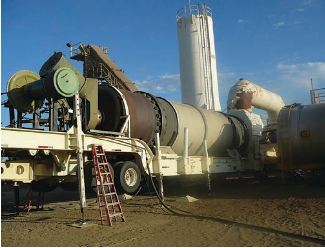
Figure 1.73. Portable parallel-flow drum plant in Baker, Montana.
