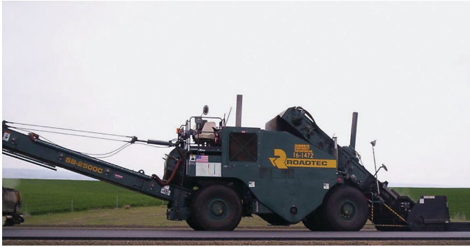
Figure 1.43. Material transfer vehicle used in Walla Walla, Washington.
