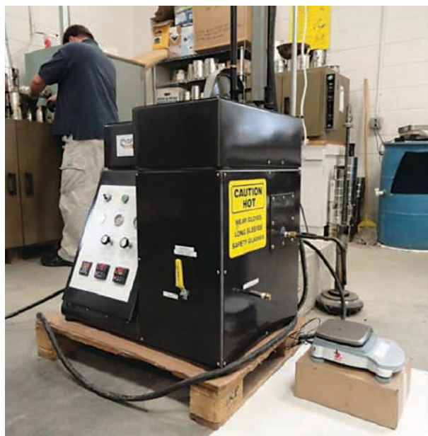
Figure 1.142. Hydrofoamer (left), polymer strained out of Florida PG 76-22 binder (right).
