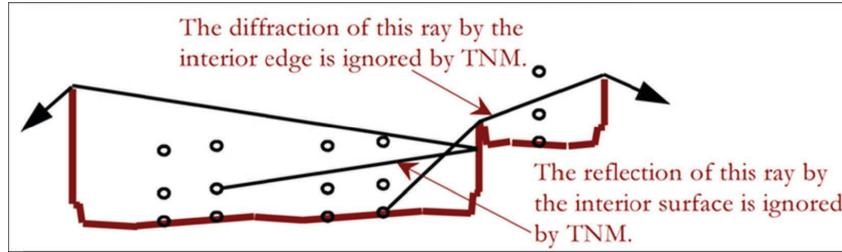
Figure 60. Text and diagram from TNM FAQs on parallel barriers.<sup>59</sup>
