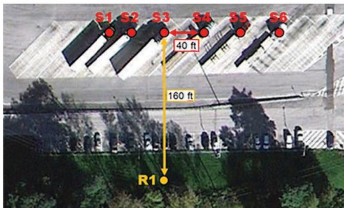
**Figure 25. Geometry for comparing array of individual noise sources to a single line source.**<sup>13</sup>
