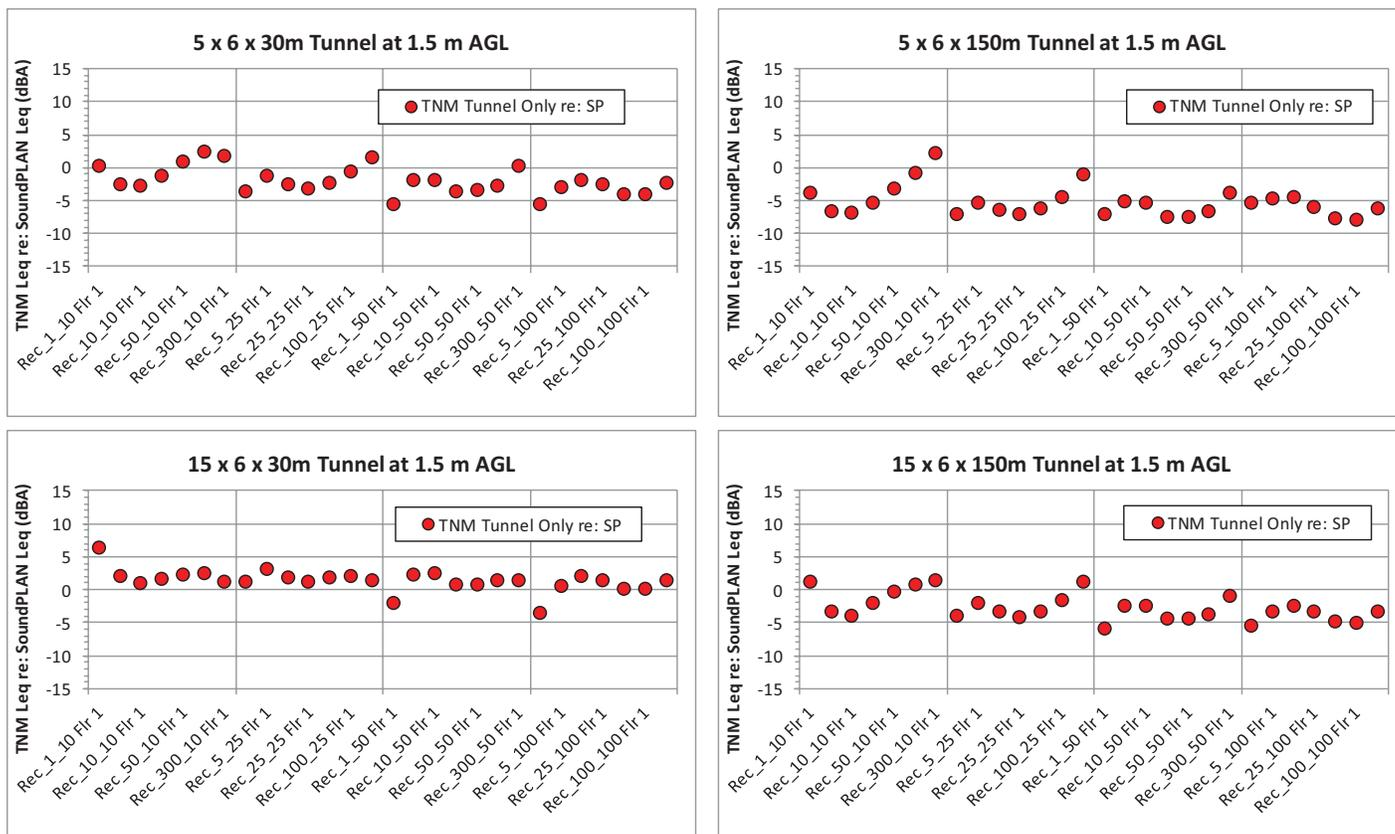
**Figure 64. TNM tunnel-only noise level minus SoundPLAN tunnel-only noise level for three parallel roads inside the tunnel, each with 1 × the volume of road outside tunnel—at distances of 1, 5, 10, 25, 50, 100, and 300 m from the tunnel opening and 10, 25, 50, and 100 m from the road centerline and 1.5 m AGL.**
