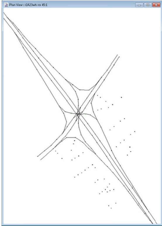
**Figure 14. FHWA TNM plan view for full modeling of an SPUI (north is to the top).**
