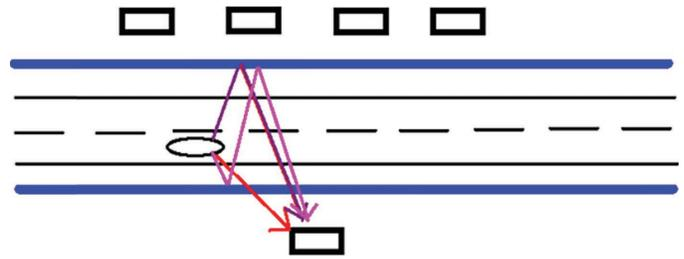
Figure 56. Plan view of multiple reflections off parallel highway noise barriers.
