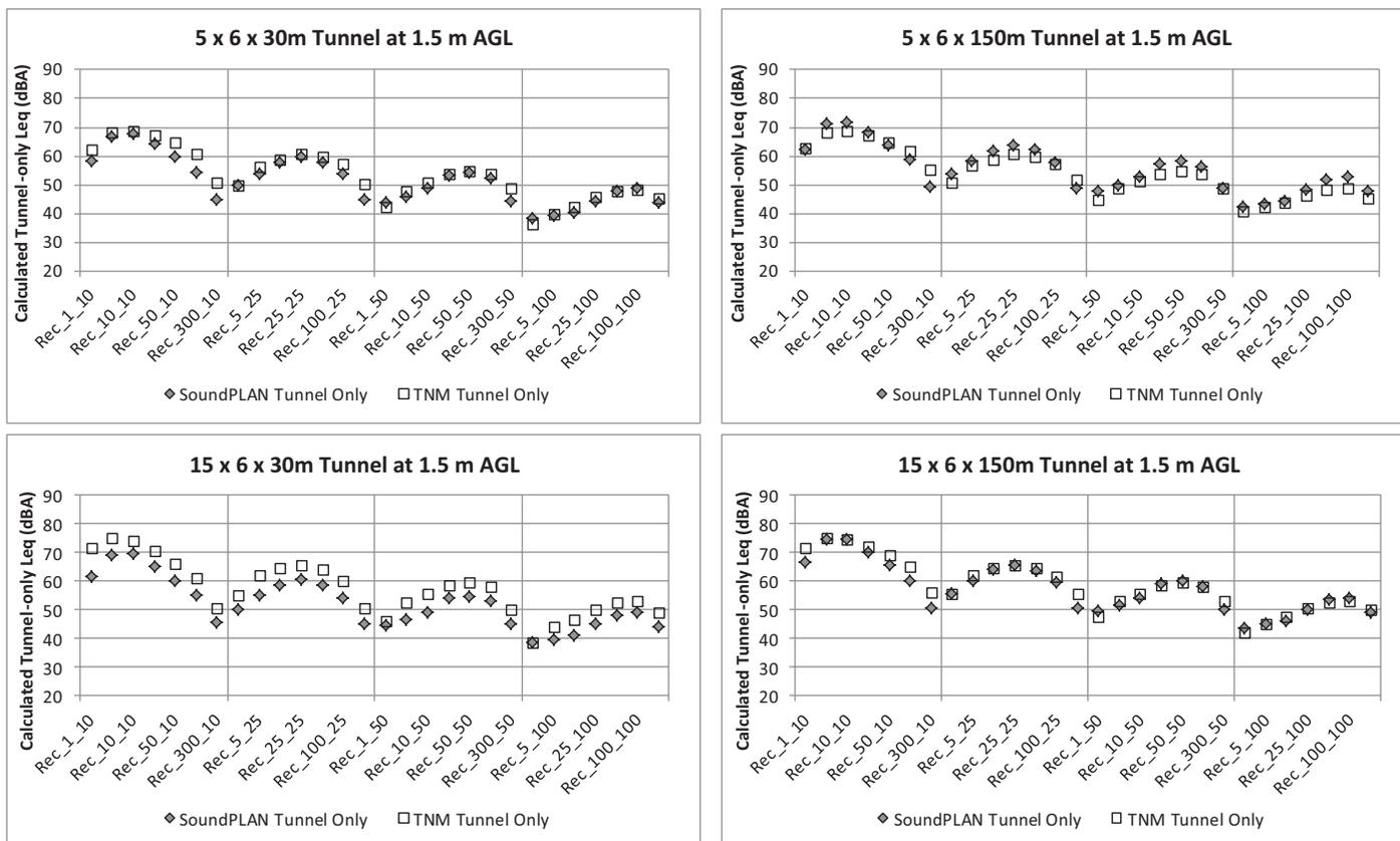
**Figure 66. TNM and SoundPLAN tunnel-only noise levels for three parallel roads inside the tunnel, each with  $2.5 \times$  the volume of road outside tunnel—at distances of 1, 5, 10, 25, 50, 100, and 300 m from the tunnel opening and 10, 25, 50, and 100 m from the road centerline and 1.5 m AGL.**
