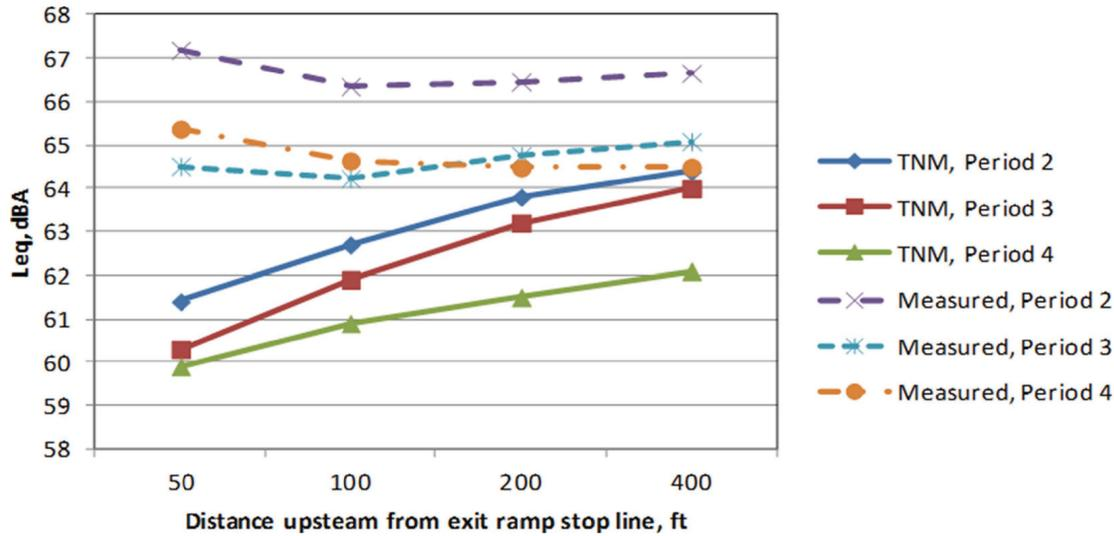
**Figure 10. Comparison of measured traffic noise and modeled noise excluding mainline heavy trucks, Briley Parkway exit ramp site.**
