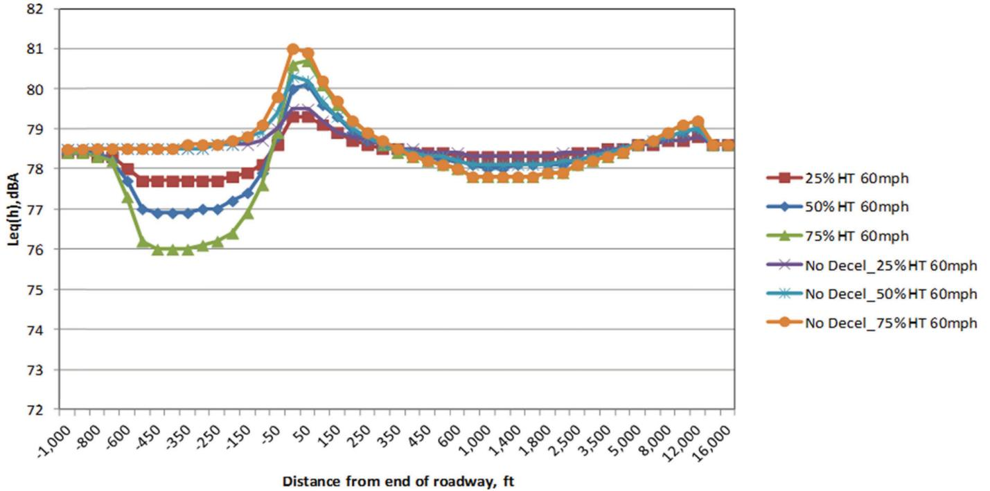
Figure 19.  $L_{eq}(h)$  for 1,000 heavy trucks for one-way “Deceleration + Cruise” compared to “All Cruise” on the upstream deceleration side for a 60-mph cruise speed and an array of receivers at a 50-ft offset distance from the roadway.
