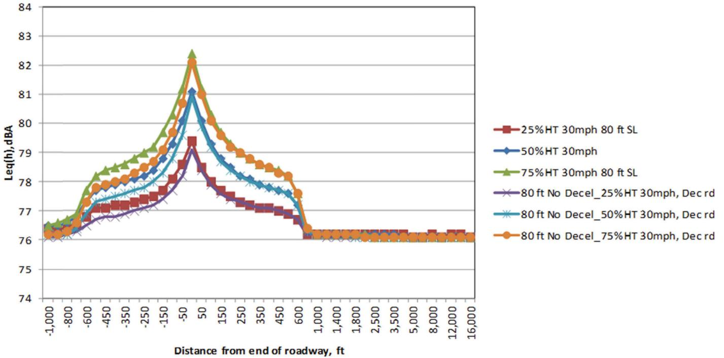
**Figure 17.**  $L_{eq}(h)$  for 1,000 heavy trucks for two-way “Deceleration + Cruise” compared to “All Cruise” on the upstream deceleration side for a 30-mph cruise speed and an array of receivers at a 50-ft offset distance from the roadway.
