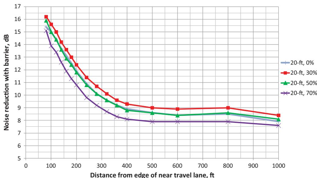
**Figure 41. Noise reduction for a 20-ft-high noise barrier along the edge of the shoulder of an eight-lane roadway with a 30-ft-high building row located 70 ft from the edge of the near travel lane, for various building percentages.**
