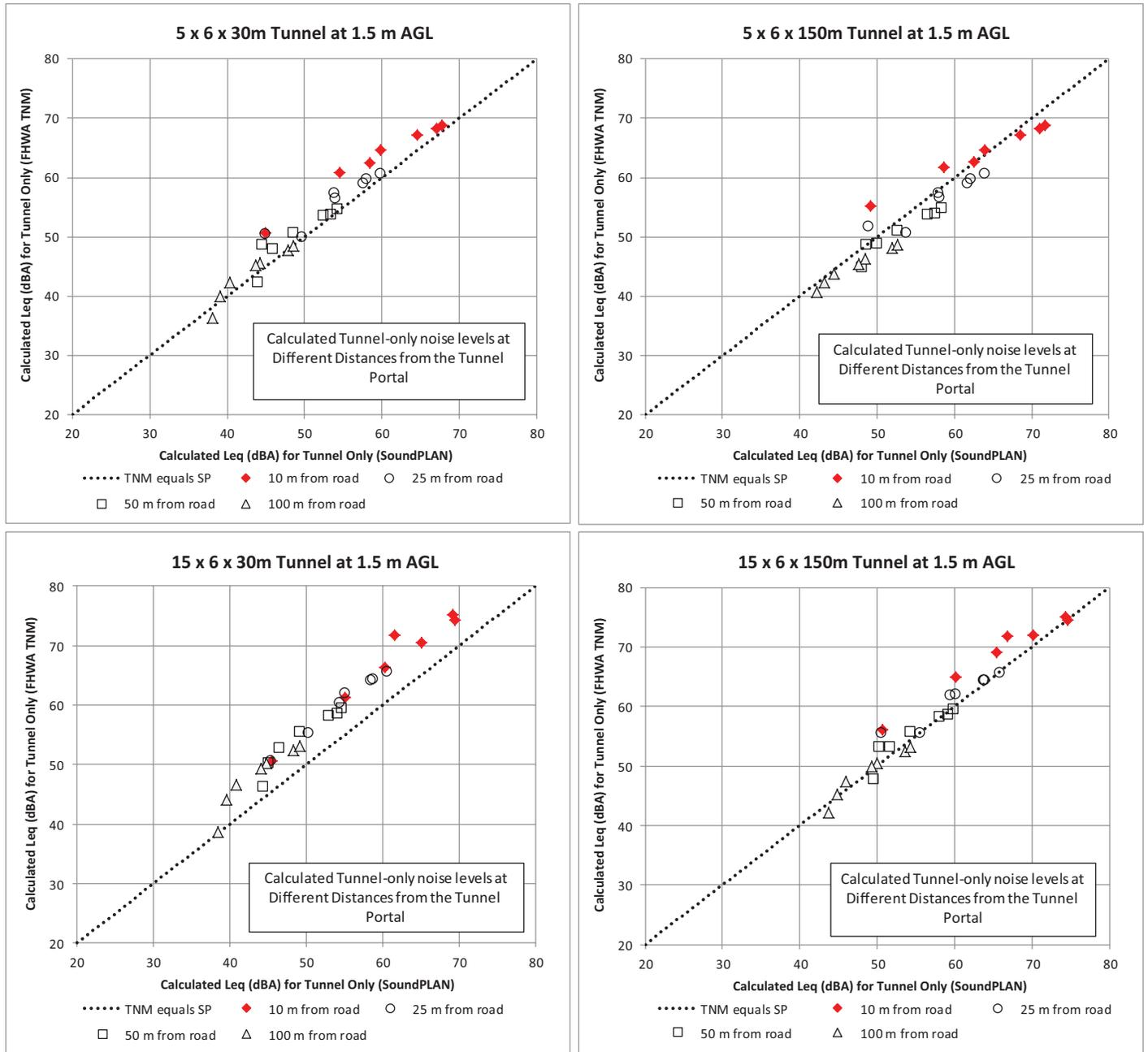
**Figure 68. FHWA TNM tunnel-only noise levels plotted against SoundPLAN tunnel-only noise levels for three parallel roads inside the tunnel, each with  $2.5 \times$  the volume of road outside tunnel—at distances of 1, 5, 10, 25, 50, 100, and 300 m from the tunnel opening and 10, 25, 50, and 100 m from the road centerline and 1.5 m AGL.**
