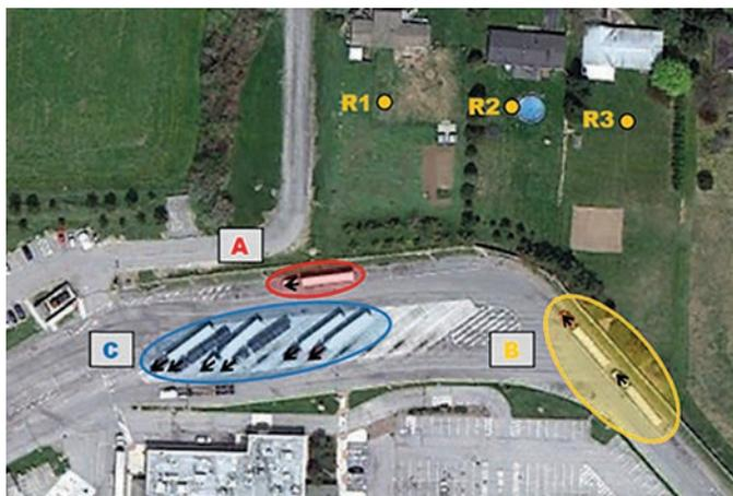
**Figure 26. Example 1—idling trucks at service plaza modeled individually.<sup>16</sup>**
