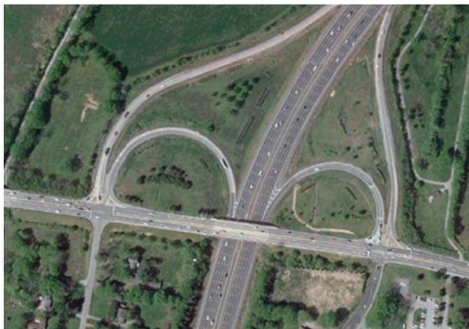
Figure 13. *Folded diamond interchange.*<sup>12</sup>
