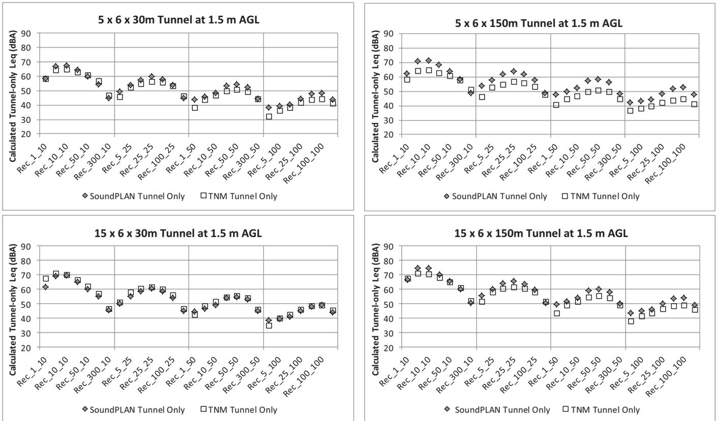
**Figure 63. TNM and SoundPLAN tunnel-only noise levels for three parallel roads inside the tunnel, each with 1 x the volume of road outside tunnel—at distances of 1, 5, 10, 25, 50, 100, and 300 m from the tunnel opening and 10, 25, 50, and 100 m from the road centerline and 1.5 m AGL.**
