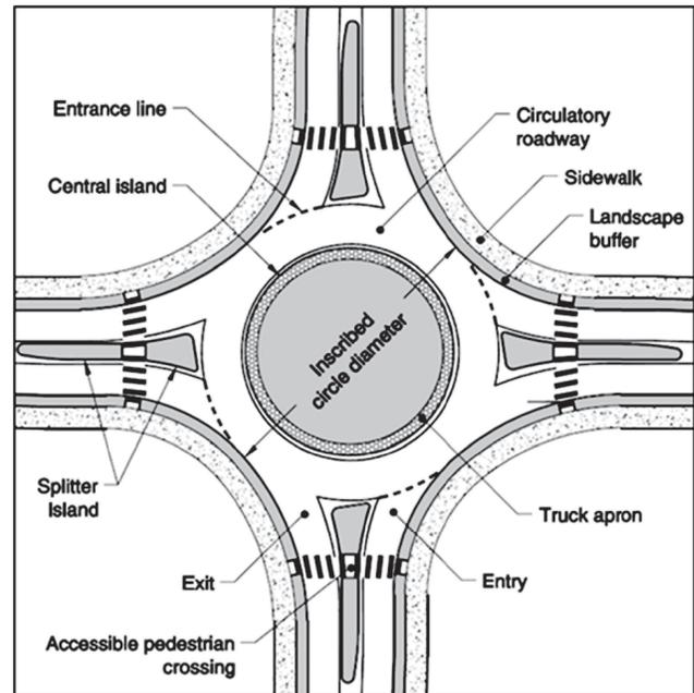
Figure 5. Modern roundabout characteristics.<sup>8</sup>
