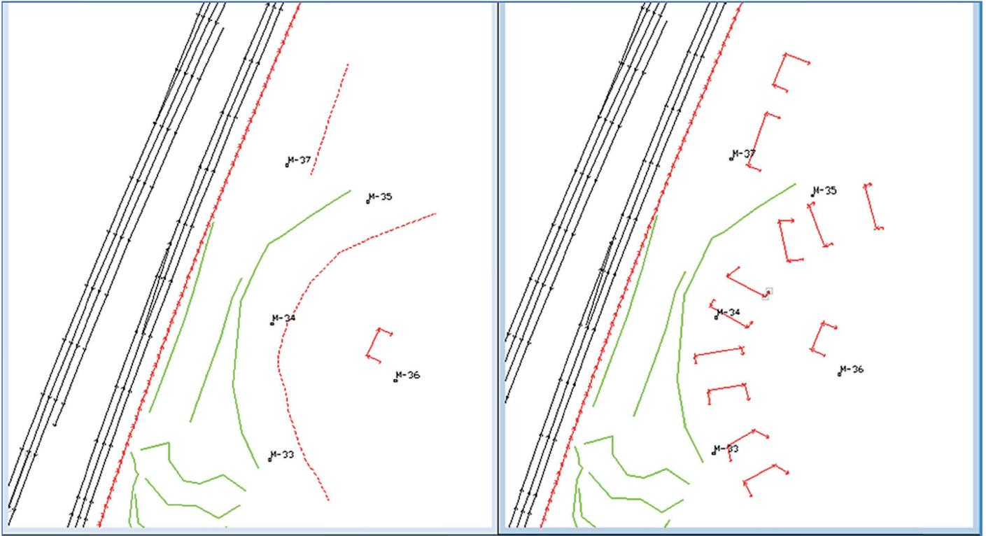
**Figure 44. TNM plan view with building rows (left) and building barriers (right), Noise Study Area G of US 29 widening.**
