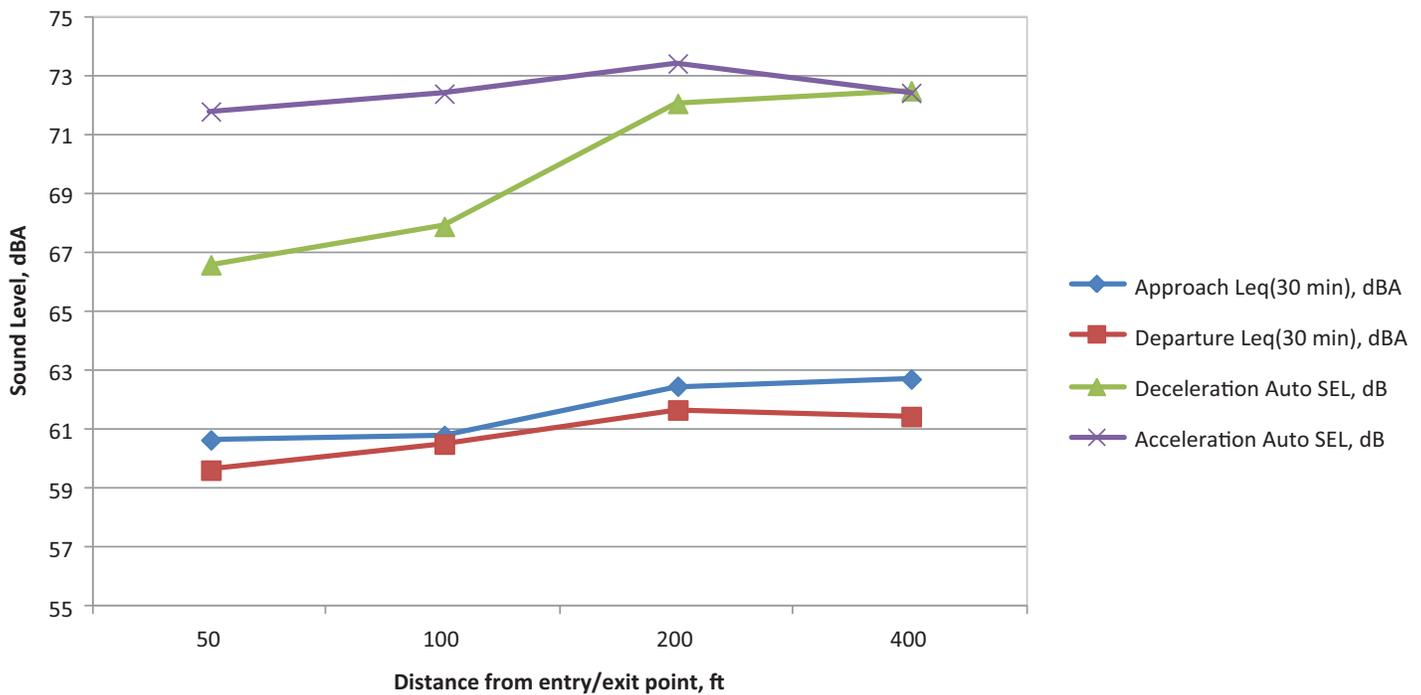
Figure 24. Measured  $L_{eq}$  (30 min) at 25-ft offset from edge of travel lane, Liberty Pike roundabout.
