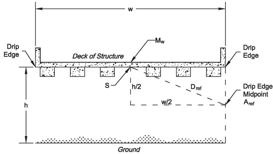
$h$  = Height of structure, from ground to underside of deck
