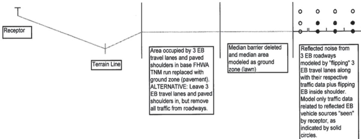
Figure 32. Skew section of reflected (flipped) FHWA TNM run.
