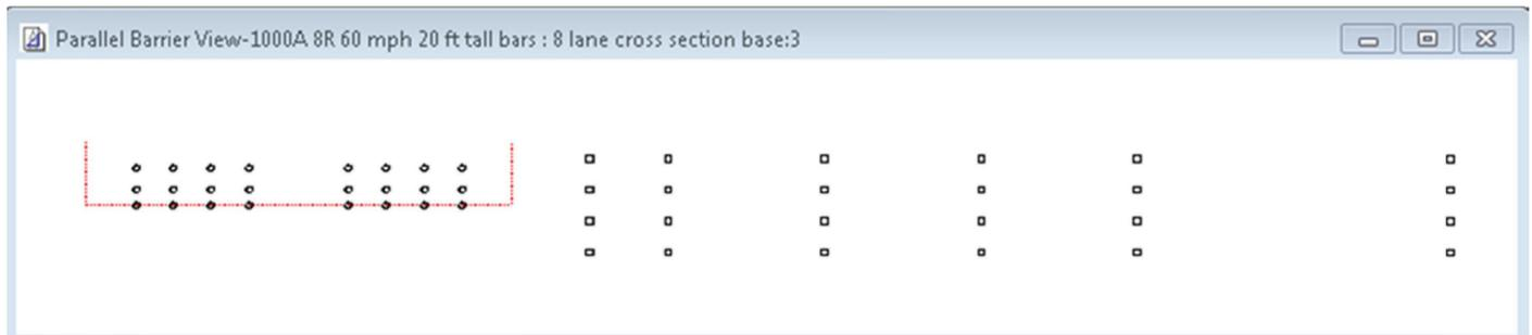
Figure 59. Illustration of receiver array at heights of 15, 5, -5 and -15 ft relative to the roadway surface and distances of 25, 50, 100, 150, 200, and 300 ft from the near wall.
