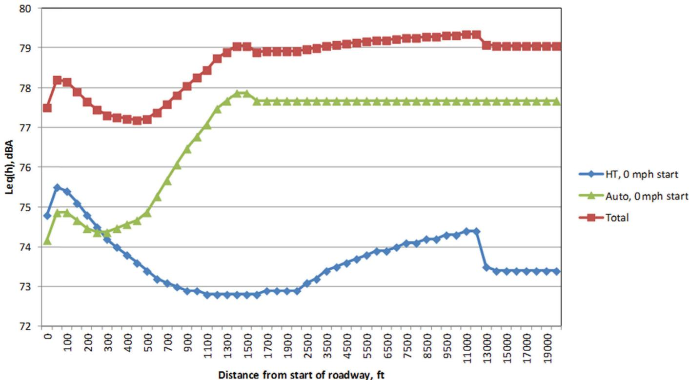
**Figure 8.**  $L_{eq}(h)$  for 97% automobiles and 3% heavy trucks (31,000 vehicles), accelerating from 0 mph to 60 mph with 100% of the Vehicles Affected and a Speed Constraint of 0 mph for a series of receivers offset 100 ft from the roadway.
