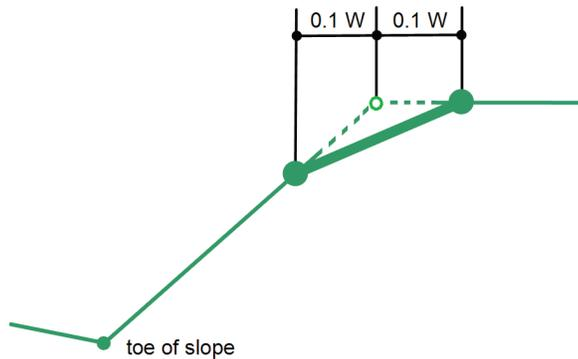
**Figure 47. Section view of flat-top berm shape including the suggested “rounding off” of the top edge.**
