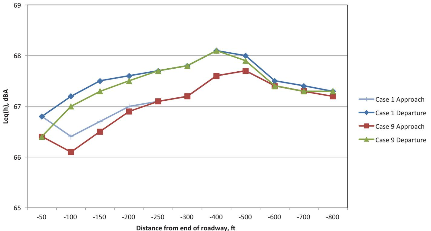
Figure 22. Comparison of  $L_{eq}(h)$  for Cases 1 and 9 for a series of receivers offset 50 ft from the western leg roadways for 1,000 automobiles approaching and departing roundabout at 40 mph.
