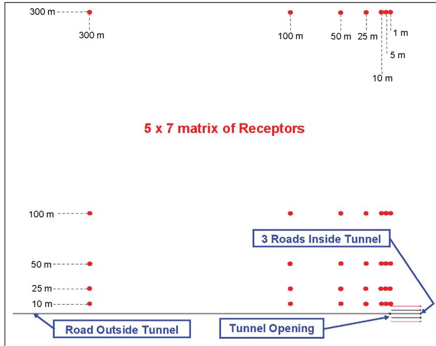
**Figure 62. Plan view of modeled geometry for tunnel measuring 15 by 6 by 30 m with three parallel and evenly spaced roads inside (with the 5-by-7 matrix of receptors).**
