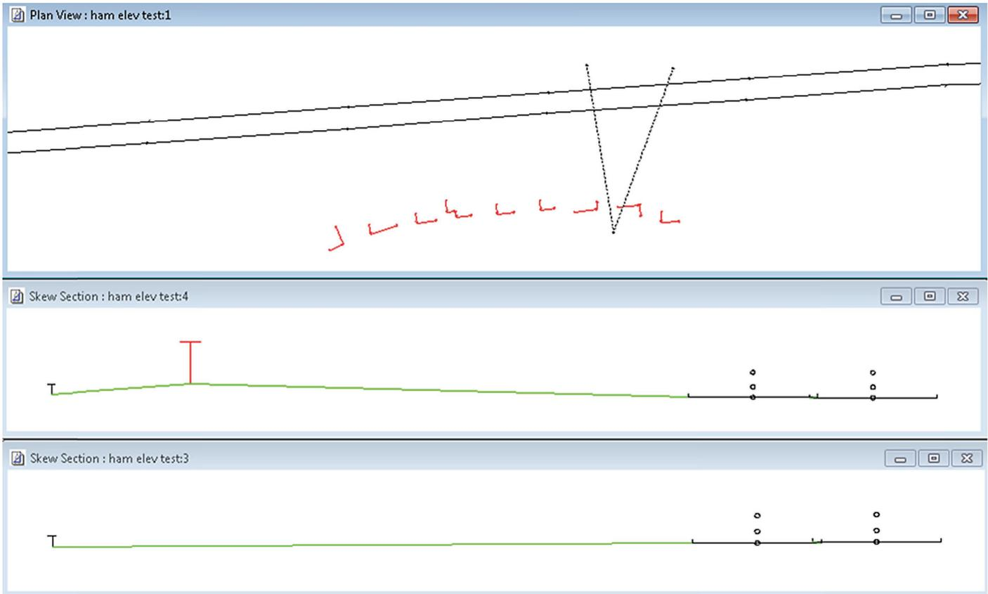
**Figure 46. FHWA TNM plan view (top) and skew section views through a building barrier (middle) and through a gap (bottom) where the ground elevation has not been defined.**
