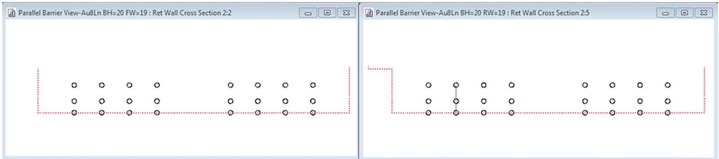
Figure 61. Cross section with 19-ft-high far wall as an external vertical surface (left) and an internal vertical surface with a 1-ft noise barrier offset 10 ft from the top of the internal vertical surface (right).
