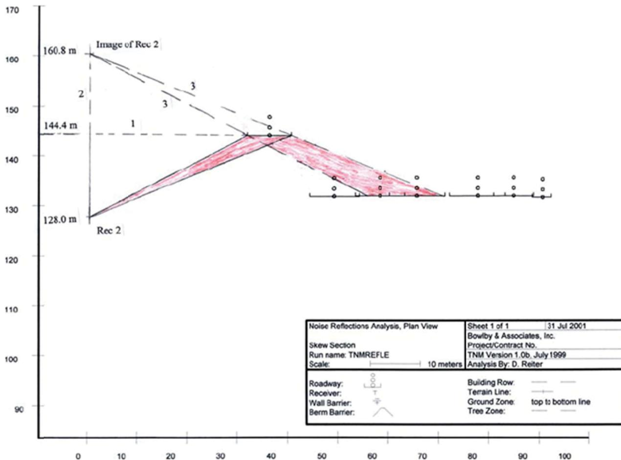
Figure 1. TNM skew section showing roadways contributing to reflected sound.<sup>2</sup>
