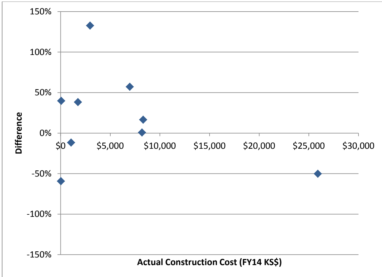
Figure 8: Case study validation – difference between predicted and actual cost
