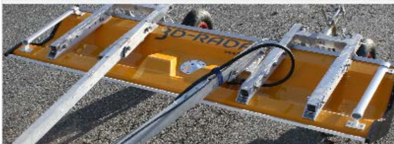
DX1821 antenna, trailer mounted.
