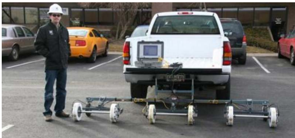
Figure C2.1. Pavement and bridge deck scanner (PBDS) towed behind a vehicle— 3 pairs of wheels at 2 feet (0.61 meter) apart.
