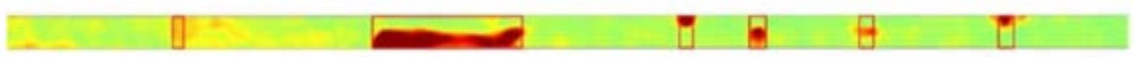
Figure B1.2. Areas of delamination based on final algorithm and statistical analysis.
