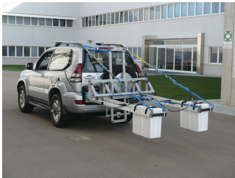
RIS Hi-Pave with two-antenna configuration.
