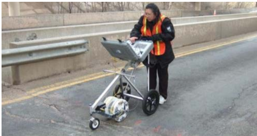
Figure C2.2. PBDS system attached to a scanning cart on asphalt overlaid bridge deck—single pair of wheels at 6 inches apart for combined impact echo/surface waves scanning.
