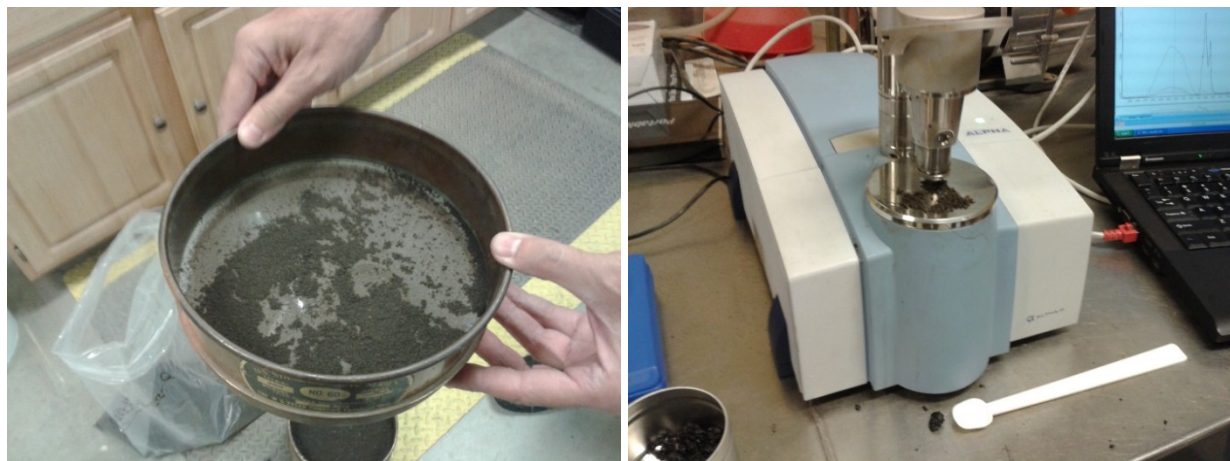
Figure B.5. Passing #30 RAP fraction (left) and ATR setup with RAP sample (right).
