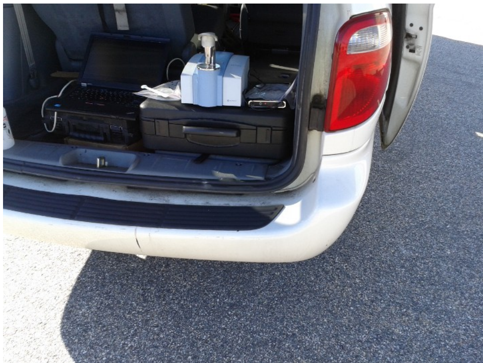
Figure B.1. ALPHA ATR FT-IR portable spectrometer set-up in the field.
