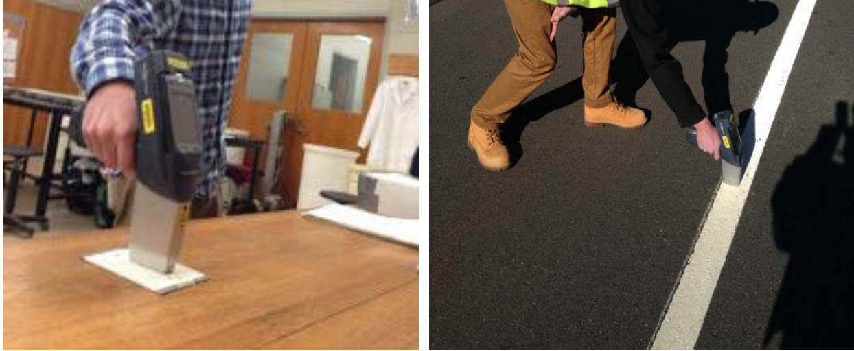
Figure B.9. XRF testing of a traffic paint control sample (left) and in situ paint strip on Exit 64, I-95, in Connecticut (right).
