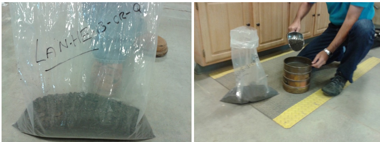
Figure B.4. Maine RAP sample in a bag (left) and sieving a RAP sample in the DOT Material Laboratory in Freeport, Maine (right).
