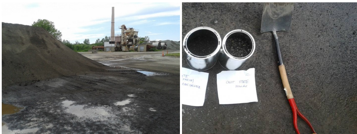
Figure B.3. RAP stockpile in Manchester, Connecticut (left), and collected RAP samples (right).
