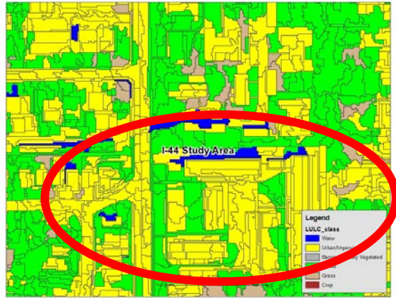
Figure 4.11. Building shadows mapped as water was a common error fixed by manual inspection (MoRAP 2014).
