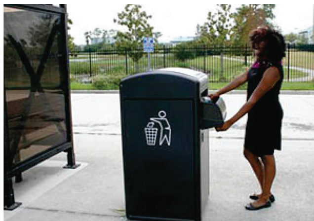
FIGURE 7 Solar trash compactors in Pinellas County, Florida, reduce the frequency of required trash removal.
