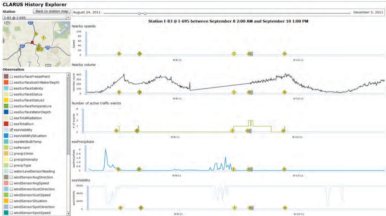
FIGURE A14 An RWIS data explorer allows an agency to see how localized weather, visibility, surface temps, etc., can affect traffic speeds, volumes, and accidents near RWIS stations.
