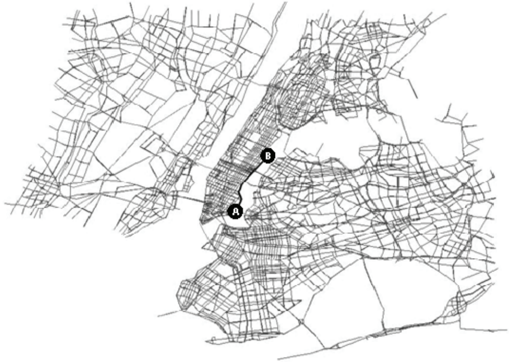
Figure 7.3. New York City network for analysis using DYNASMART-P. (Points A and B delineate the path along which travel time distributions were examined in Manhattan.)
