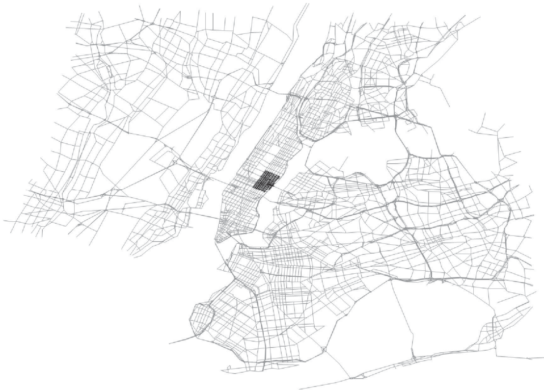
Figure 8.1. Study networks: DYNASMART-P New York City network (gray) and Aimsun Manhattan network (black).
