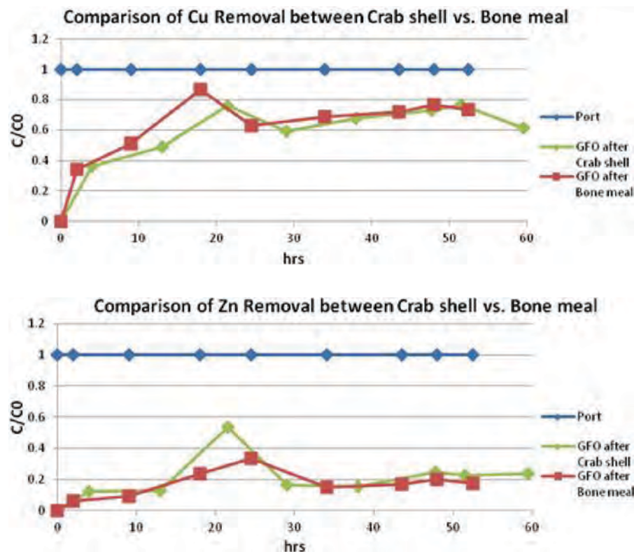
Figure 5-31. Comparing the effects of crab shell and bone meal on copper and zinc removal in a FBR.
