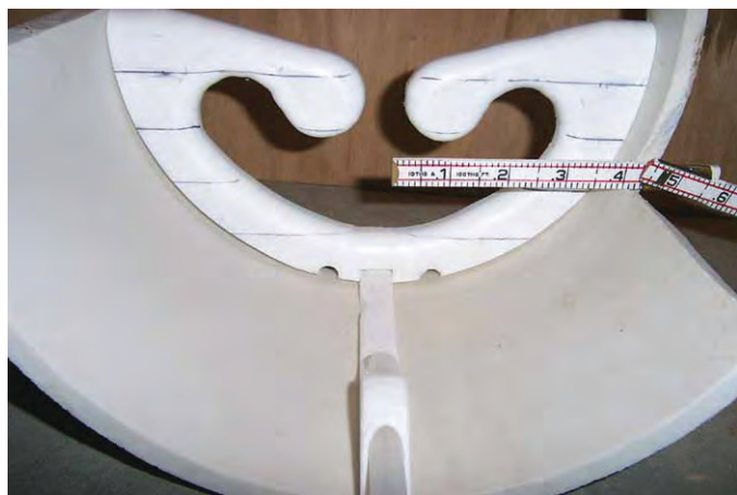
Figure 2. Static mixer (from Smith and Granato (2010)).
