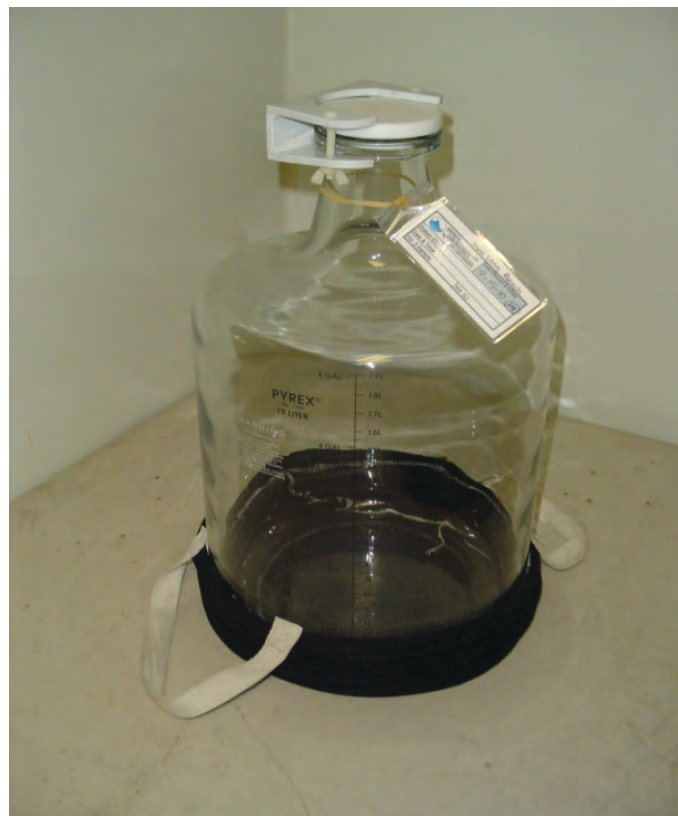
Figure 4. Composite bottle showing bottle bag used for transport and lifting.
