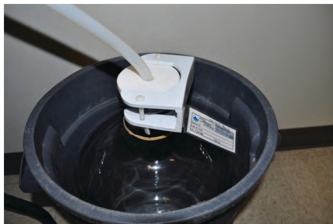
Figure 3. Composite bottle with label and installed tubing.
