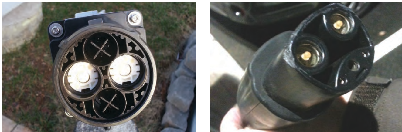
FIGURE 5 Level 3 connectors: (Left) CHAdeMO connector; (Right) Tesla Supercharger. Note: The SAE combo connector, a third type of Level 3 connector, is not shown. (Source: LeighFisher January 2014.)
