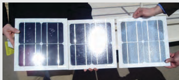
Left: smooth float glass; Middle: glass with anti-reflective coating; Right: deeply textured glass Photo credit: Cliff Ho, Sandia National Laboratories; PV samples from Canadian Solar, Inc.
