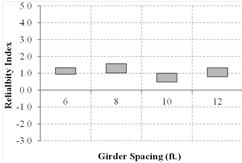
Figure 5-3 Reliability Indices Of Various Bridge Decks Designed Using A 1.0 Live Load Factor Over A 1 Year Return Period (ADTT=5000), Positive Moment Region, Class 2 Exposure
