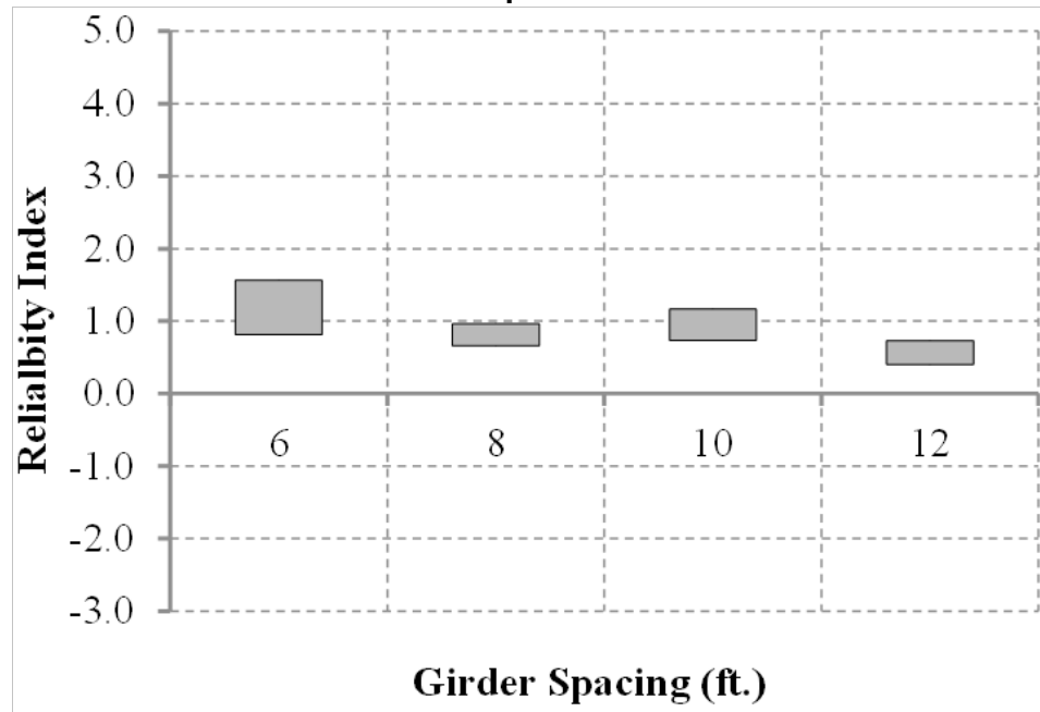
Figure 5-4 Reliability Indices Of Various Bridge Decks Designed Using A 1.0 Live Load Factor Over A 1 Year Return Period (ADTT=5000), Negative Moment Region, Class 2 Exposure
