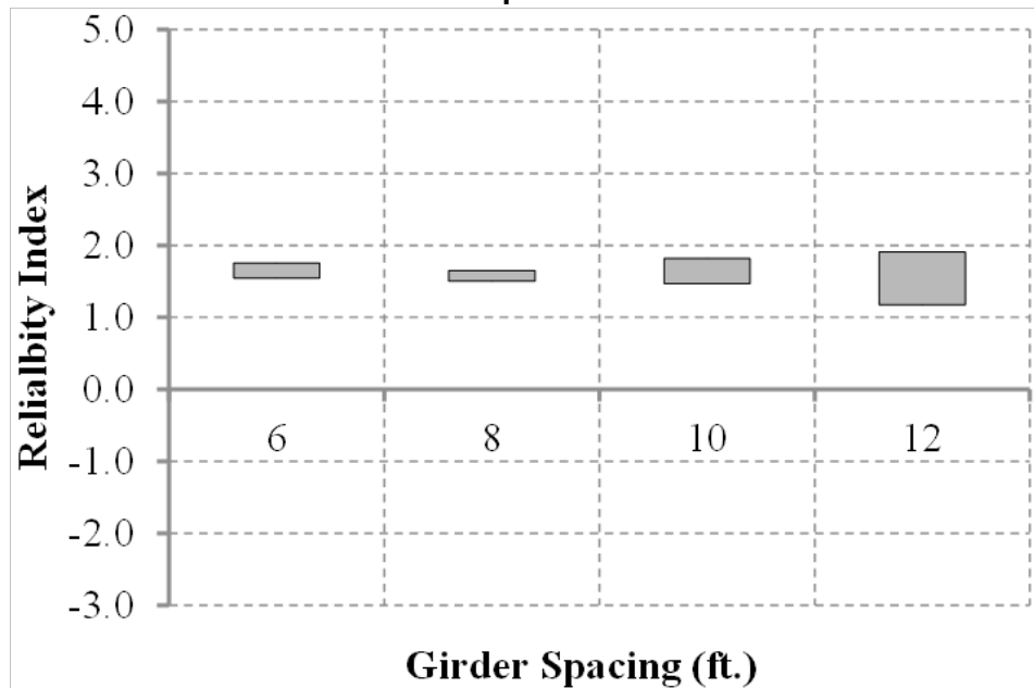
Figure 5-2 Reliability Indices Of Various Bridge Decks Designed Using A 1.0 Live Load Factor Over A 1 Year Return Period (ADTT=5000), Negative Moment Region, Class 1 Exposure
