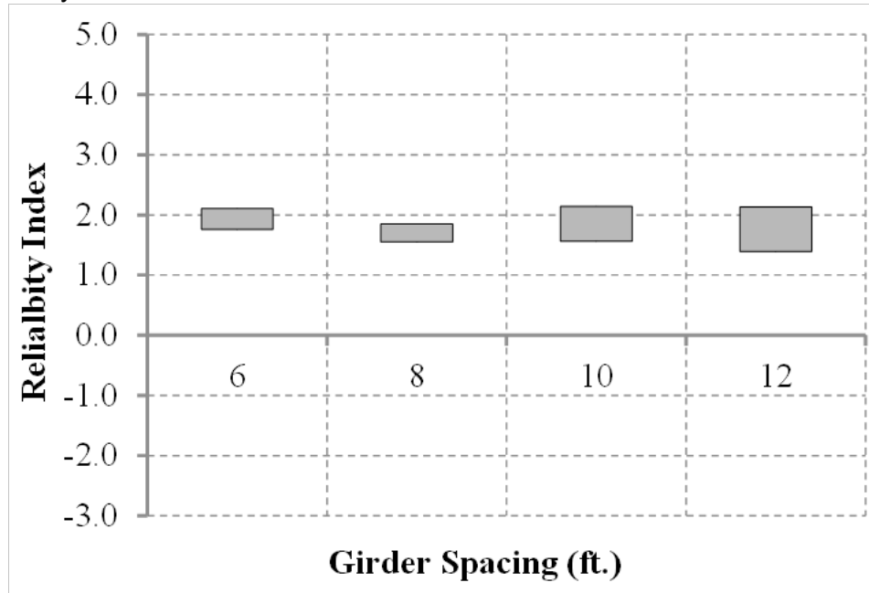
Figure 5-1 Reliability Indices of Various Bridge Decks Designed Using a 1.0 Live Load Factor Over A 1 Year Return Period (ADTT=5000), Positive Moment Region, Class 1 Exposure
