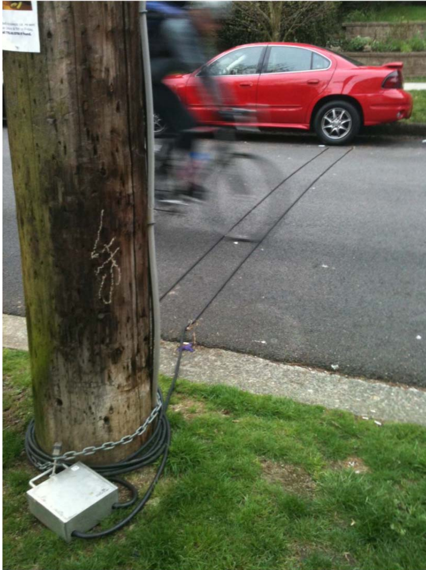
FIGURE 5 Pneumatic tube bicycle counter in Vancouver, British Columbia. (Image: Jean-Francois Rheault, Eco-Counter; used with permission.)
