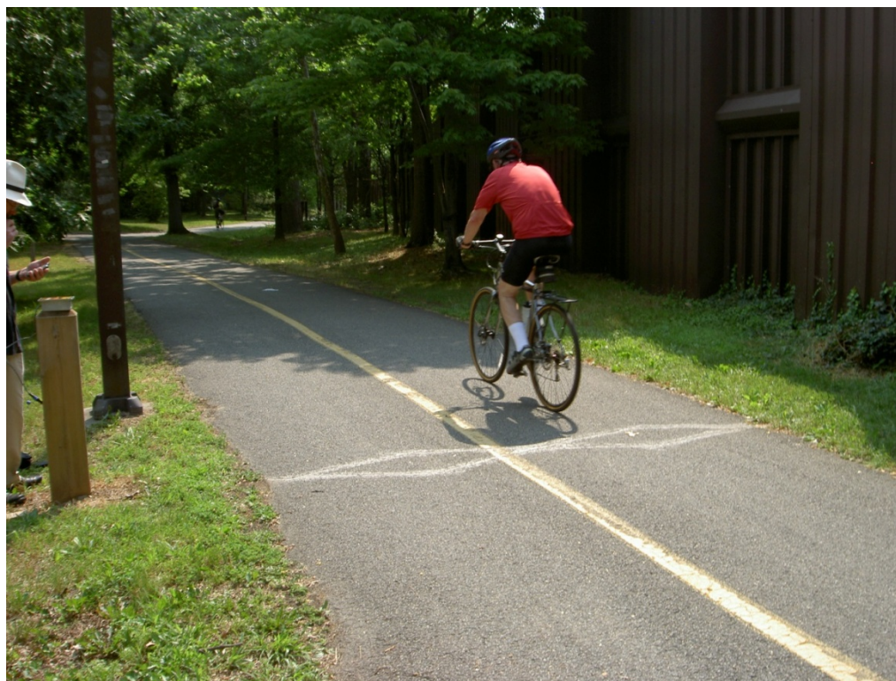
FIGURE 6 Permanent counter on a shared-use path in Arlington, Virginia, with an inductance loop in the pavement and the infrared counter and processing unit hidden in the wooden post at left. (Image: Krista Nordback, P.E., Ph.D.; used with permission.)
