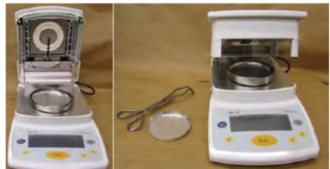
FIGURE 39 Sartorius Model MA 150 1,200-g moisture analyzer (Berney et al. 2011).
