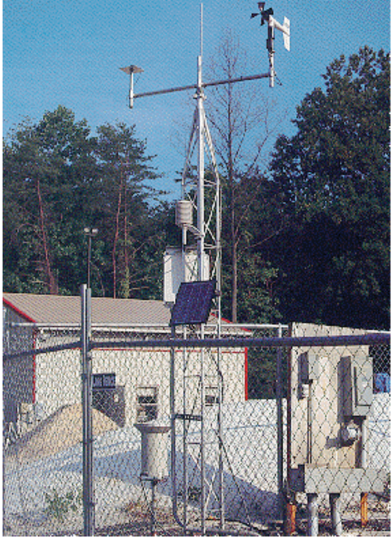
Figure 4.19. Road weather information system at the Turner–Fairbank Highway Research Center. Source: Zaccagnino (1996).
