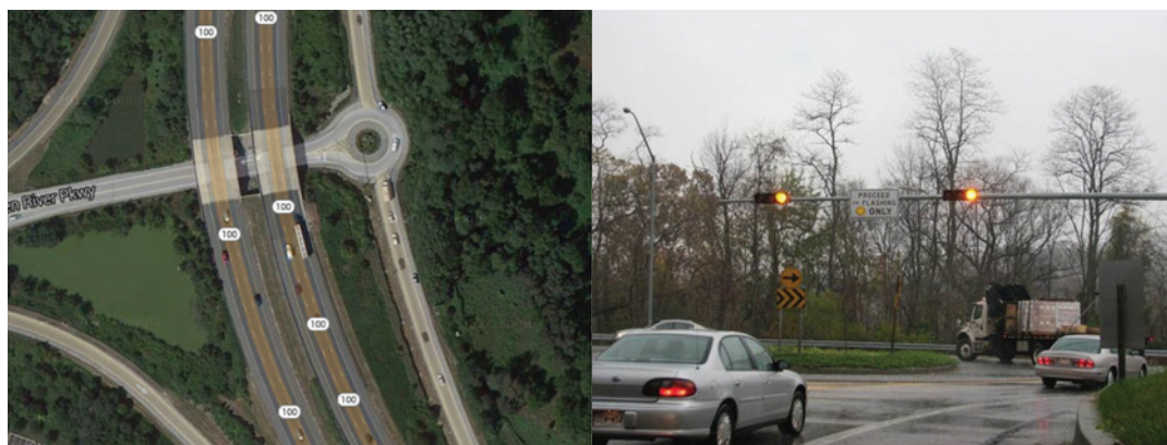
Figure 3.21. (a) Aerial image of Maryland roundabout and (b) photo showing the signalized arterial leg of the roundabout.
