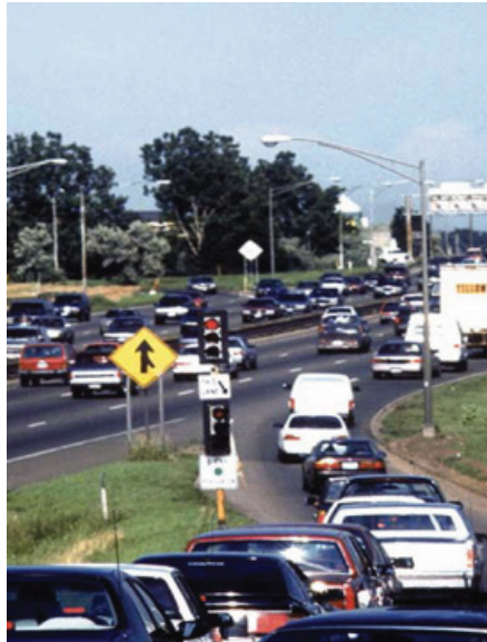
Figure 4.14. Ramp meter. Source: FHWA (2004).
