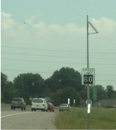
Figure 4.15. Variable speed limit sign in Missouri.
