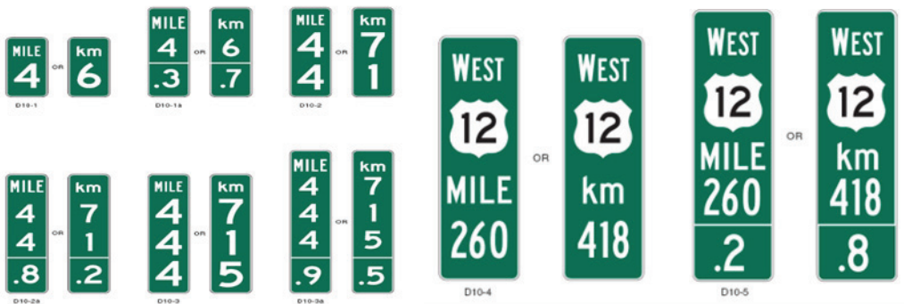
Figure 4.18. Examples of highway reference markers. Source: MUTCD (FHWA 2009).
