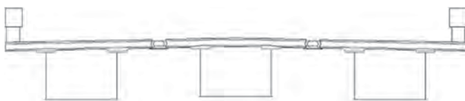
Figure A.22. Three adjacent box girder units.
