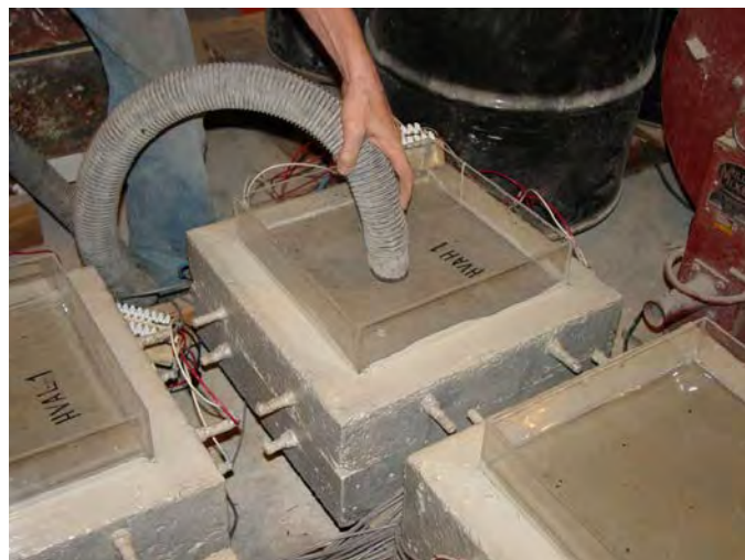
Figure F.19. Vacuuming off the water at the end of the wet period.
