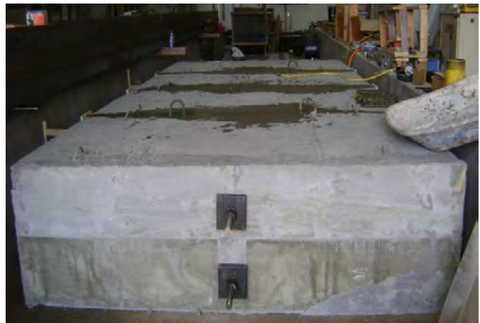
Figure C.14. Specimen after grouting shear keys.
