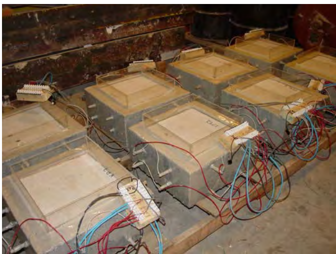
Figure F.17. Specimens ready to start the wet-dry cycle.
