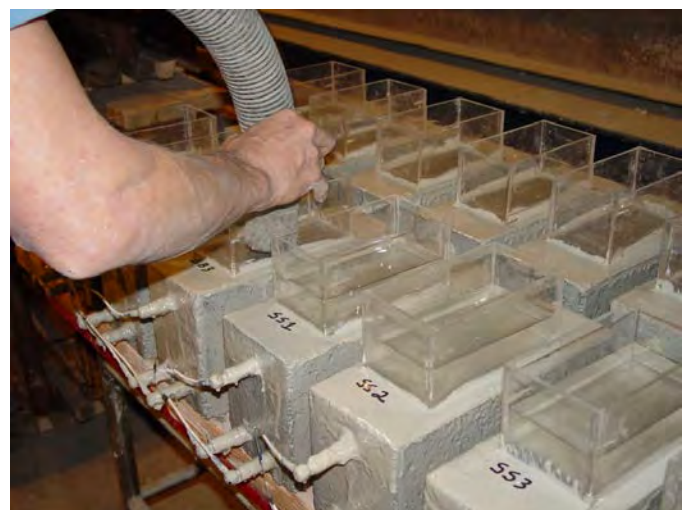
Figure E.14. The salt solution was removed by vacuuming after the wet period was finished.
