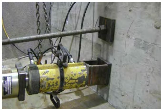
Figure C.15. Jacking the specimen to AASHTO specifications.
