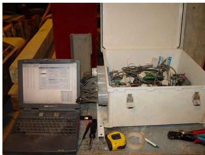
Figure F.20. Laptop and data logger system used to collect the data.
