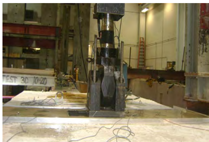
Figure C.18. Actuator at interior joint for bottom tension setup.
