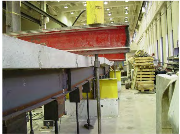
Figure 3.94. Large deformation due to yielding of bottom flange at midspan.
