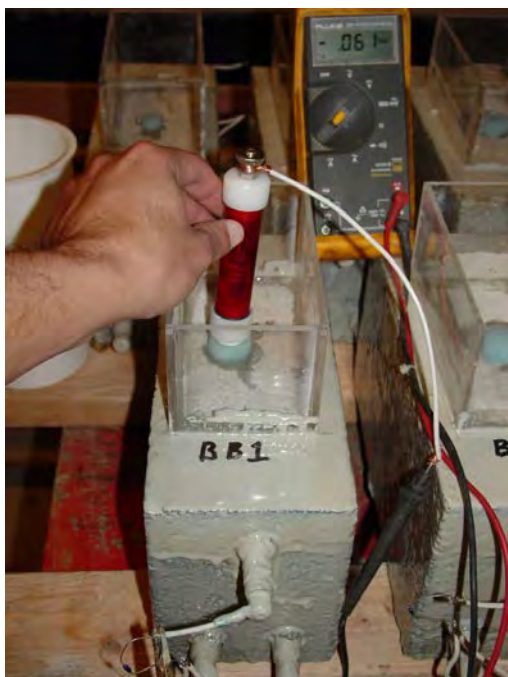
Figure E.15. Measuring the half-cell potential.
