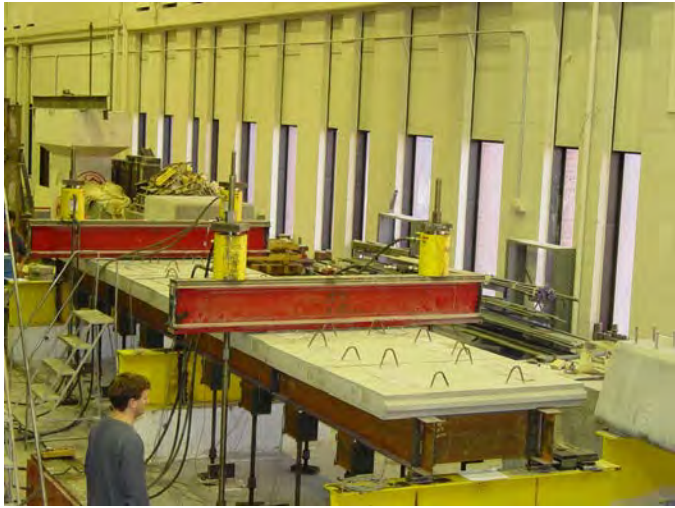
Figure 3.89. Ultimate load test setup.
