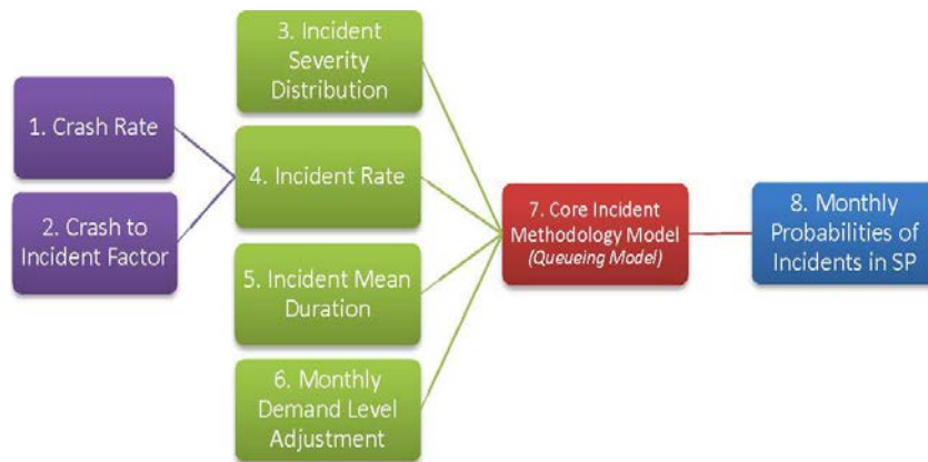
Figure F.1. Proposed data structure for estimating incident probabilities in a data-poor environment.
