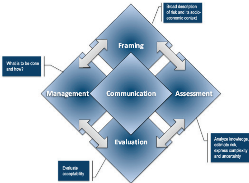
FIGURE A8-6 Components of the risk governance framework. SOURCE: Adapted from Anonymous, 2008.
