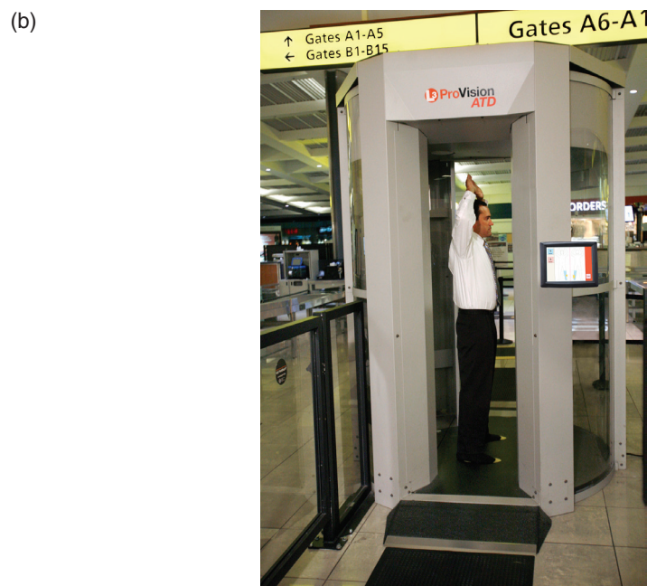
FIGURE 1.1 Advanced imaging technologies deployed by TSA: (a) X-ray-based Rapiscan Secure 1000. (b) Millimeter-wave-based L-3 ProVision ATD. SOURCE: (a) Courtesy of Scott Olson/Getty Images; (b) Courtesy of L-3 Communications.
