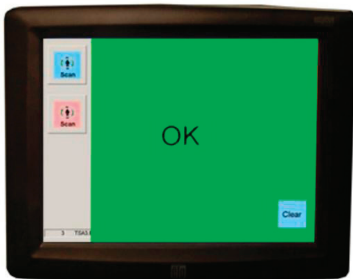
FIGURE 1.3 Images from a millimeter wave AIT equipped with automatic target recognition. NOTE: If potential threat items are detected on the person being scanned, they are indicated on a generic outline of a person that is identical for all passengers screened (a). Areas identified as containing potential threats will require additional screening. (b) If no potential threat items are detected, an “OK” appears on the monitor with no outline. SOURCE: Courtesy of the Transportation Security Administration.
