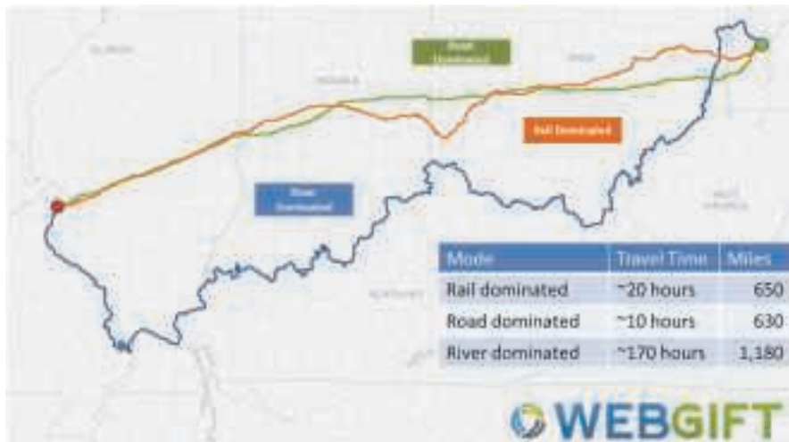
FIGURE G-1 Dominant modal routes and characteristic distances and travel times for transport between Pittsburgh and Saint Louis.
