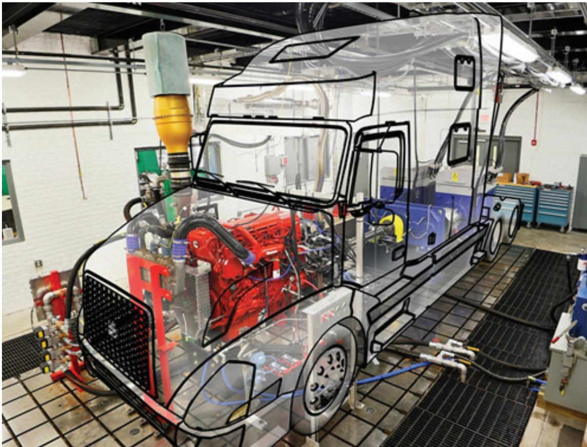
**FIGURE 4-3** 500 kW dynamometer with diesel engine-under-test in ORNL VSI Laboratory with truck outline overlay. SOURCE: Smith et al. (2014).
