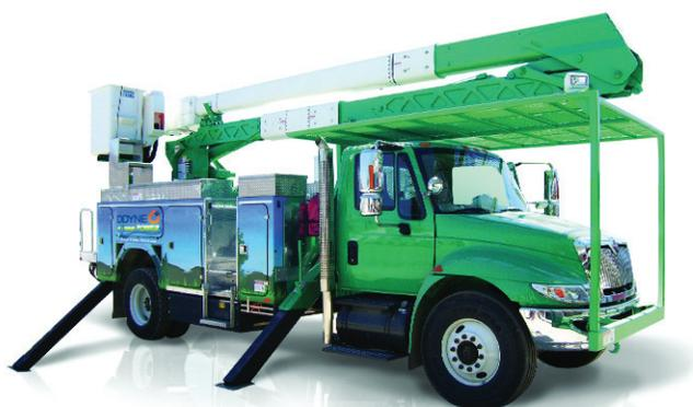
**FIGURE 4-1** Odyne Class 6 plug-in hybrid utility lift truck. SOURCE: Green Fleet Magazine (2008). Courtesy of Odyne Systems, LLC.
