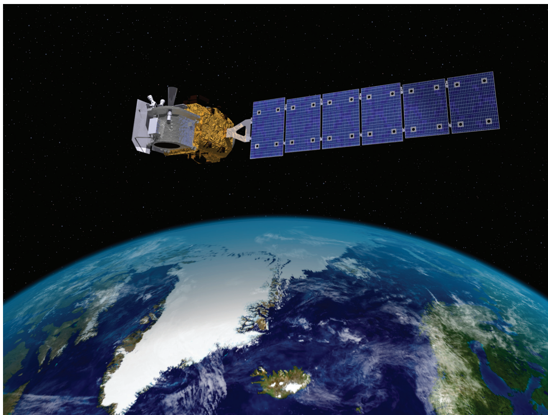
FIGURE 3.2.1 The Ice, Cloud, and land Elevation Satellite-2 (ICESat-2) is the second generation of the laser altimeter ICESat mission and is scheduled for launch in July 2016. SOURCE: Courtesy of Orbital ATK.
