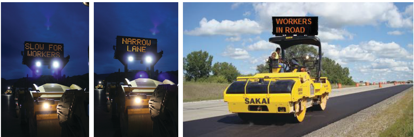
FIGURE 52 PCMS mounted on pavement roller: night (left) and day (right) (Pappe 2014).
