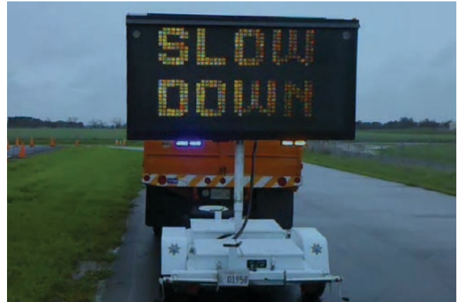
FIGURE 12 PCMS augmented with flashing “police” lights (Ravani 2012).
