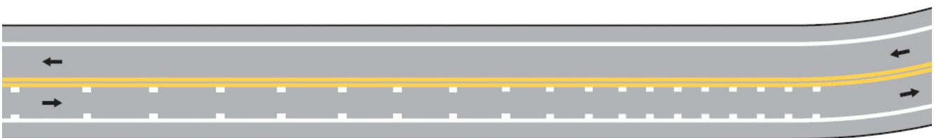
FIGURE 30 Peripheral transverse bar markings application diagram from the U.S. MUTCD (FHWA 2009).
