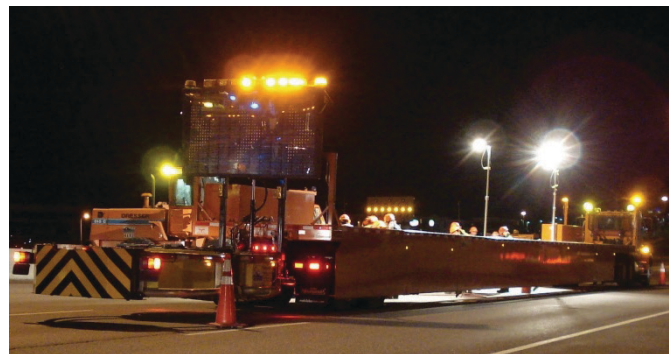
FIGURE 24 Balsi beam ( left ) and MBT-1 ( right ) (Caltrans 2004, Mobile Barriers LLC 2014).
