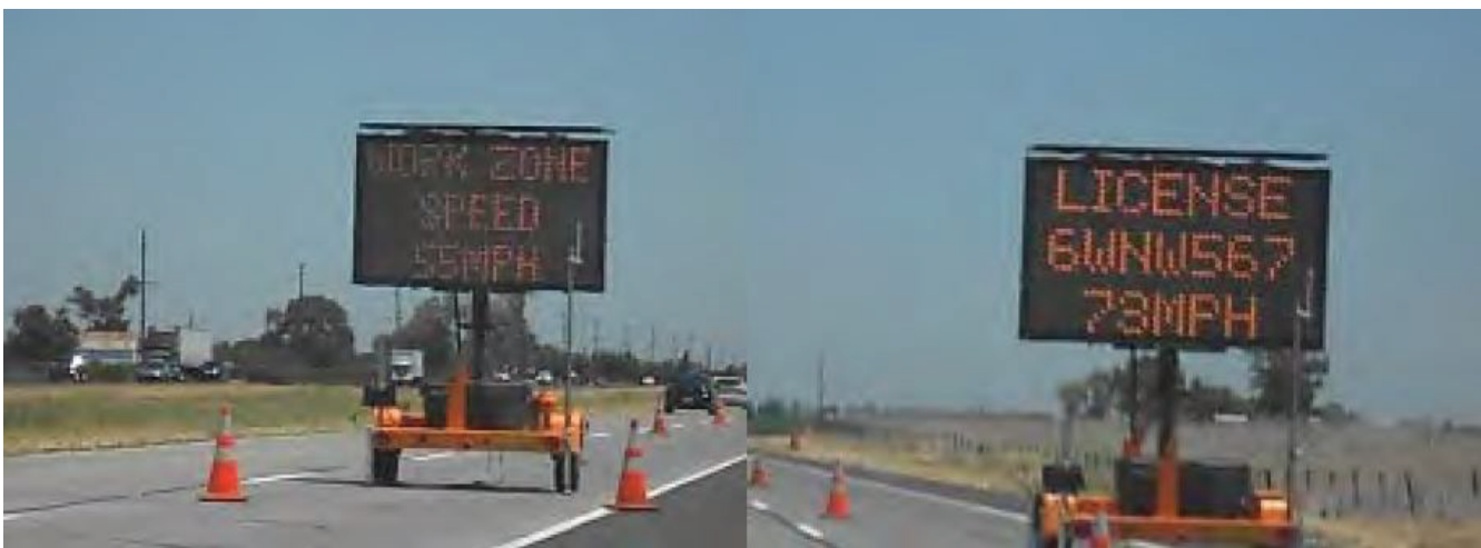
FIGURE 14 Messages displayed to speeders by the augmented enforcement system (Chan et al. 2013).
