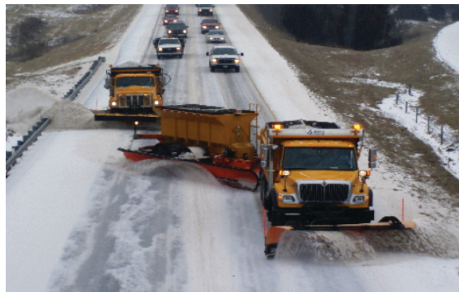
FIGURE 32 Although not typically intended as a speed control measure, snow removal operations often result in situations where traffic is “paced” by maintenance vehicles (Viking-Cives 2014).
