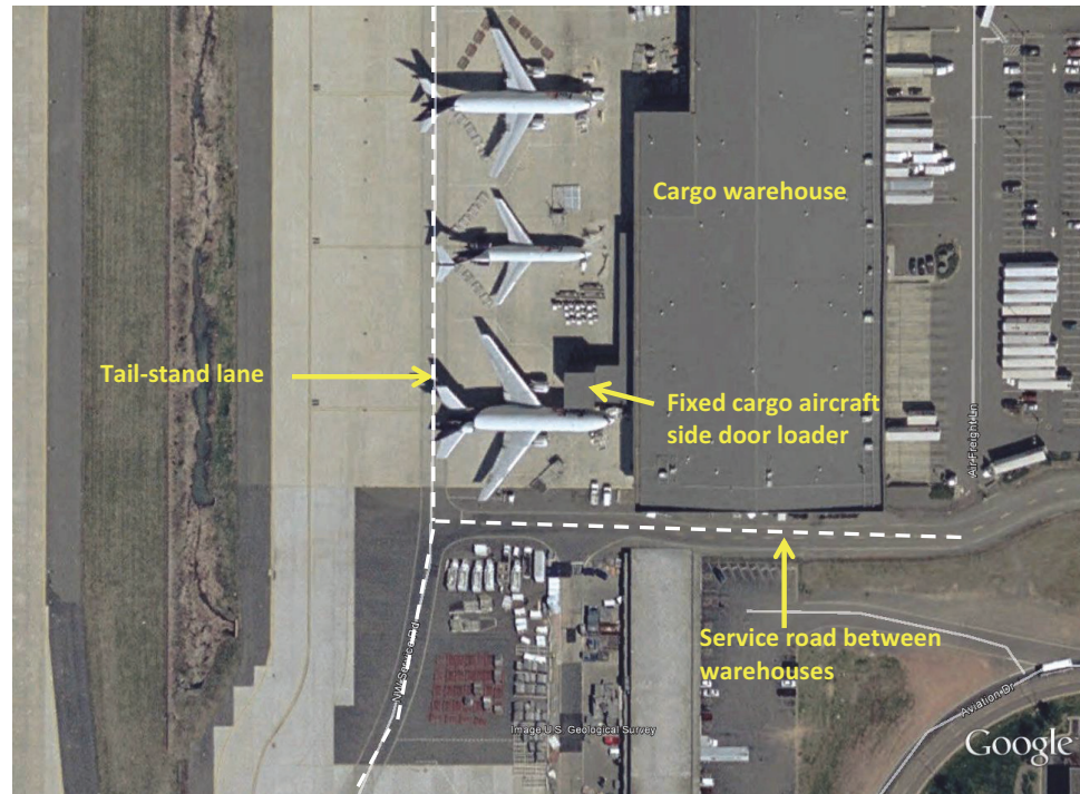
Figure 4-10. Roads between cargo buildings and apron configuration.
