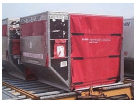
(ii) Lower Deck Container
