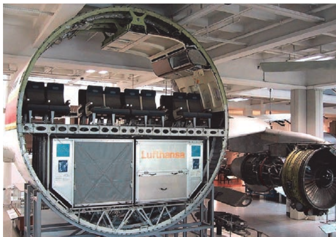
Figure 2-3. Airbus A300 aircraft cross-section displaying cargo containers on lower deck.
