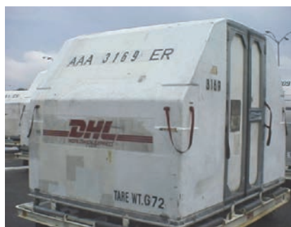
(i) Upper Deck Container
