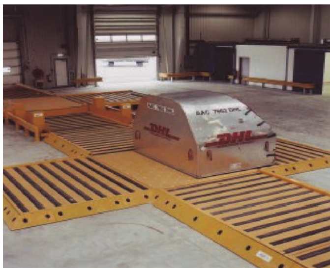
Figure 4-14. Moderately mechanized sort-and-load example.
