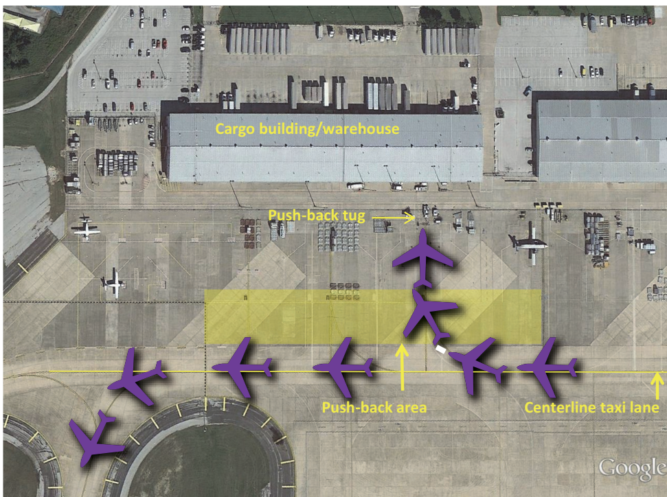
Figure 4-5. Air cargo apron push-back area and process.
