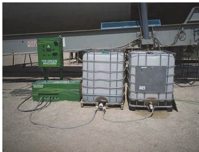
Figure A-26. WMA foaming system at the Wyoming field site.
