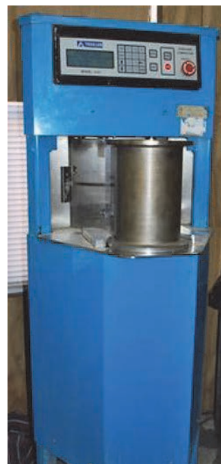
Figure A-9. Troxler compactor used to prepare the on-site PMLC specimens.
