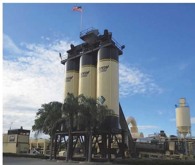
Figure A-42. Duval asphalt DBG drum plant in Jacksonville, Florida.
