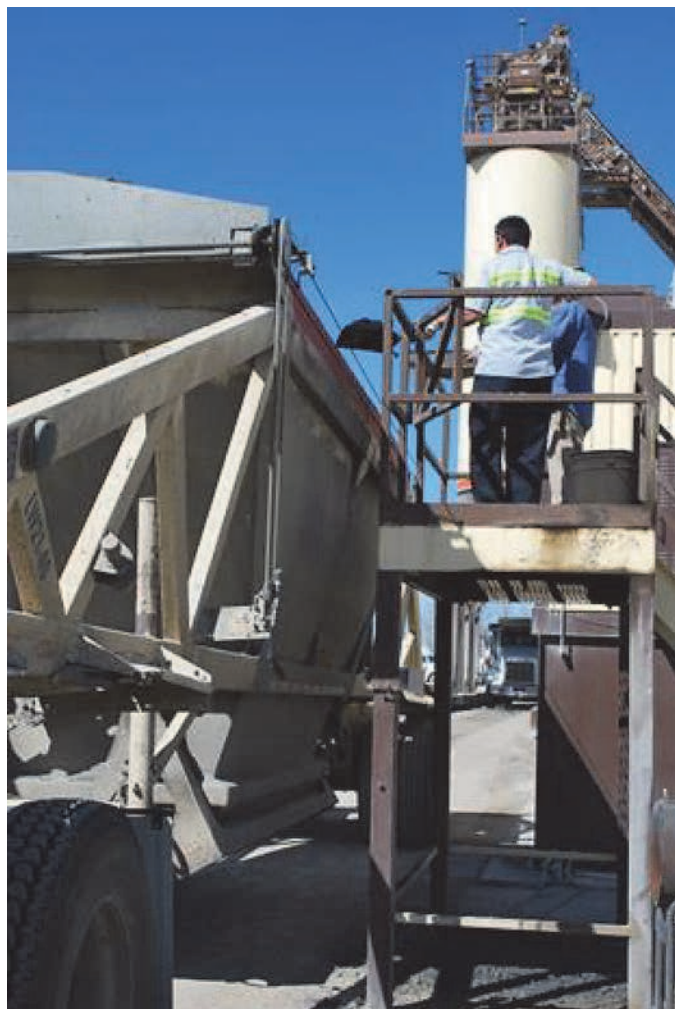
Figure A-8. Loose mix collection from the truck at RTI hot mix plant.
