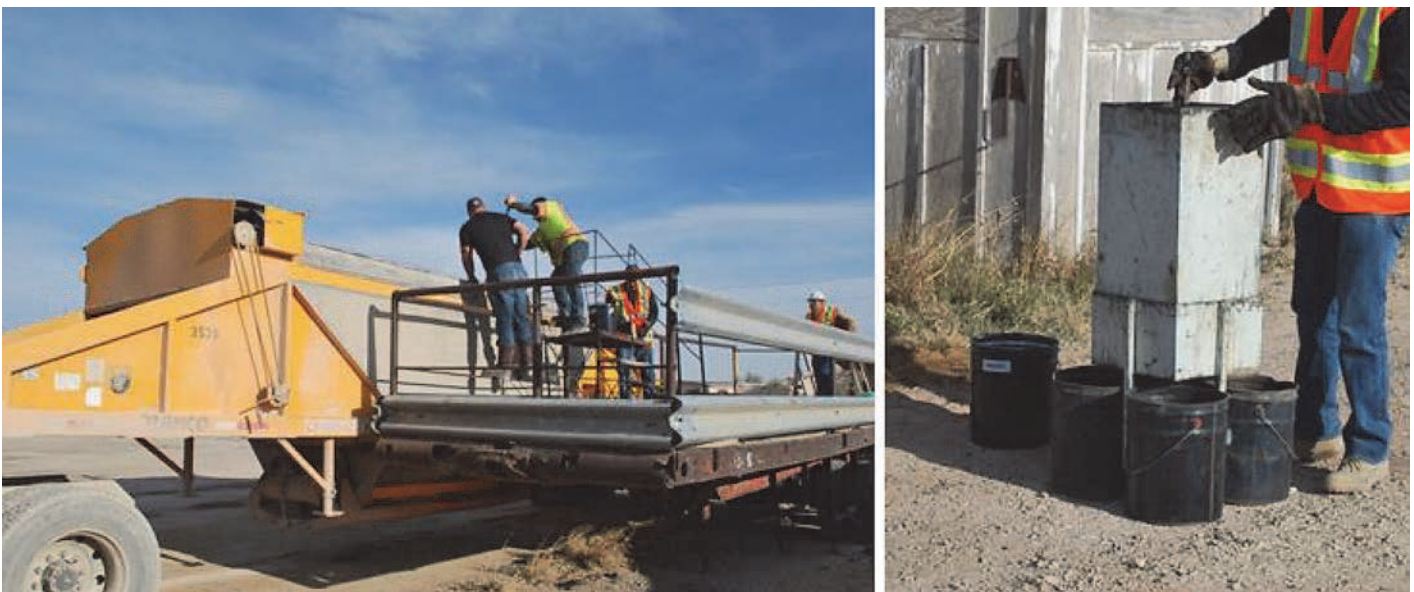
Figure A-65. Loose mix sampling from truck in Midland–Odessa batch plant.
