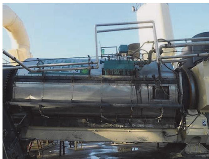
Figure A-43. DBG multiple-nozzle foaming manifold used in Jacksonville, Florida.
