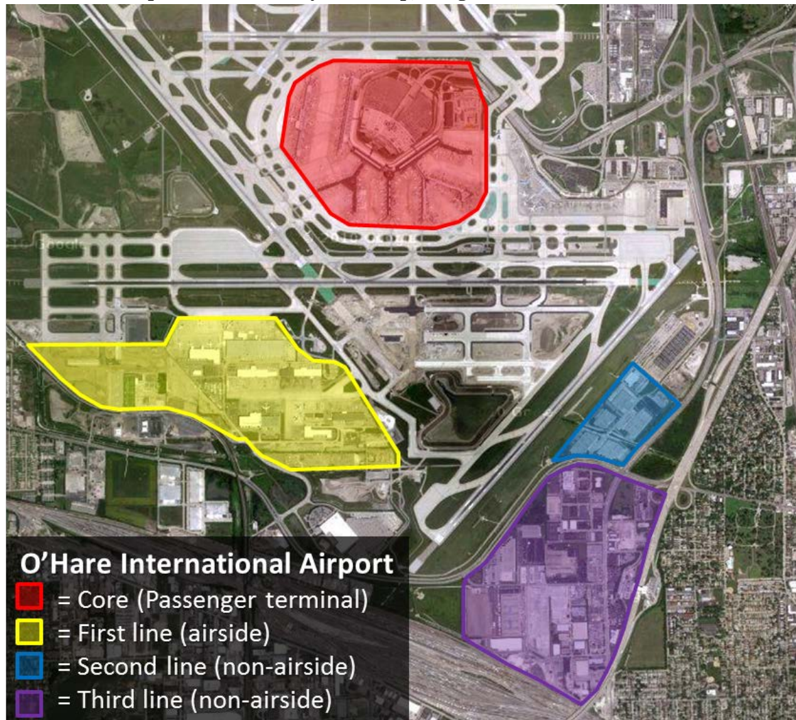
Figure 4-9 First Line, Second Line, and Third Line Air Cargo Facilities at Chicago O’Hare International Airport. (SOURCE: Lynxs Group, Google Earth Pro)
