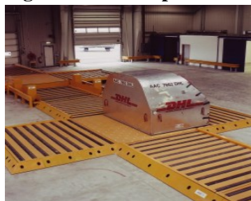
Figure 9-26 Examples of Moderately Mechanized Sort and Load. (SOURCE: CDM Smith.)
