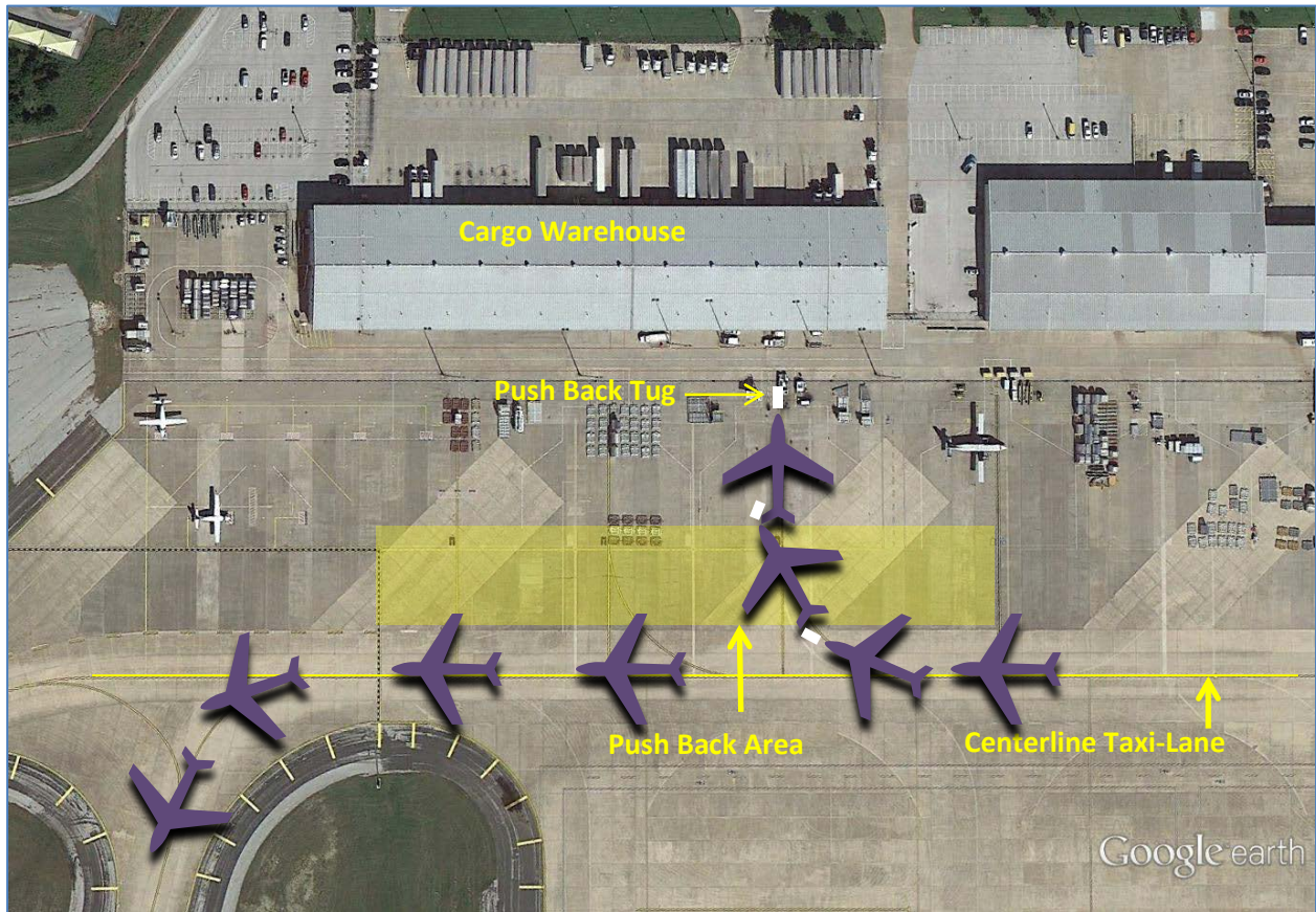
Figure 9-20 Air Cargo Apron Push Back Area and Process. (SOURCE: Google Earth Pro, CDM Smith Analysis.)
