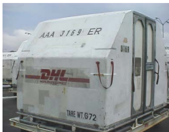
(i) Upper Deck Container
