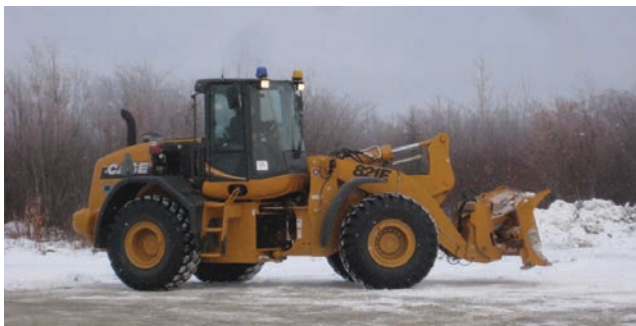
FIGURE 22 Typical articulated front-end loader with attachments used at Alaskan rural airports. Photo credit: J. Worrall, Alaska DOT&PF.
