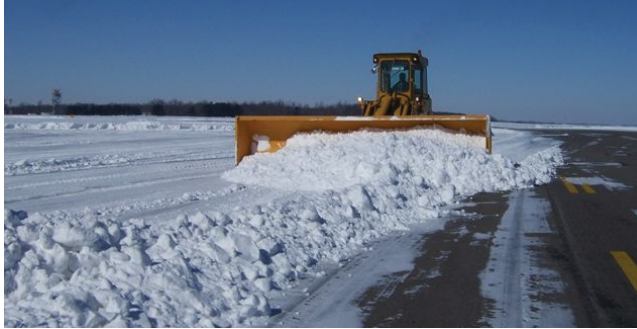
FIGURE 9 Example of a frontend loader with ramp plow moving a large volume of snow. Photo credit: M. Daugherty, Mansfield, Ohio.
