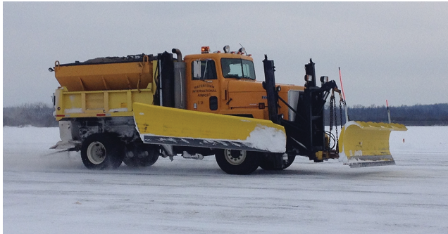
FIGURE 6 Typical snowplow vehicle with front blade, bat wing plow, and sand spreader. Photo credit: G. Sussey, Watertown, New York.
