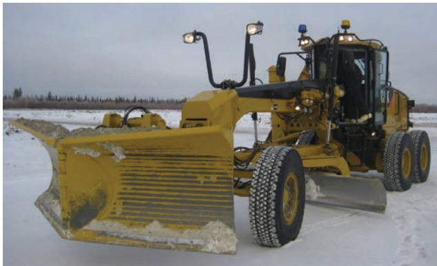
FIGURE 21 Typical grader with underbody and front plow used at Alaskan rural airports. Photo credit: J. Worrall, Alaska DOT&PF.
