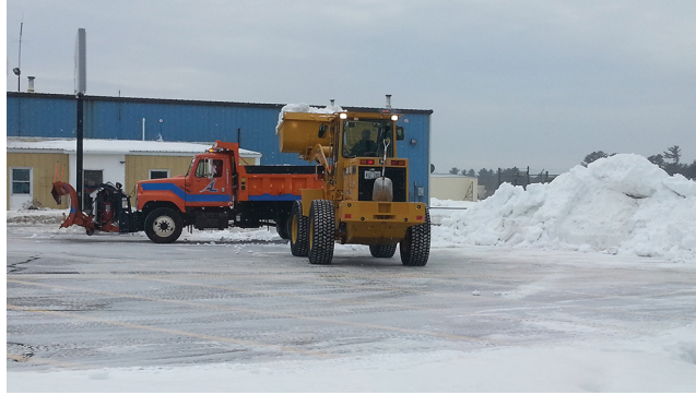
FIGURE 15 Example of a front-end loader removing snow mounds. Photo credit: R. Lanham, Auburn, Maine.
