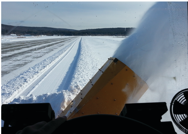
FIGURE 8 View of snowblower removing a plowed windrow. Photo credit: M. Moriarty, Keene, New Hampshire.
