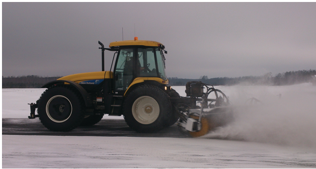
FIGURE 7 Typical multi-purpose tractor vehicle with sweeper attachment. Photo credit: R. Horn, Eagle River, Wisconsin.
