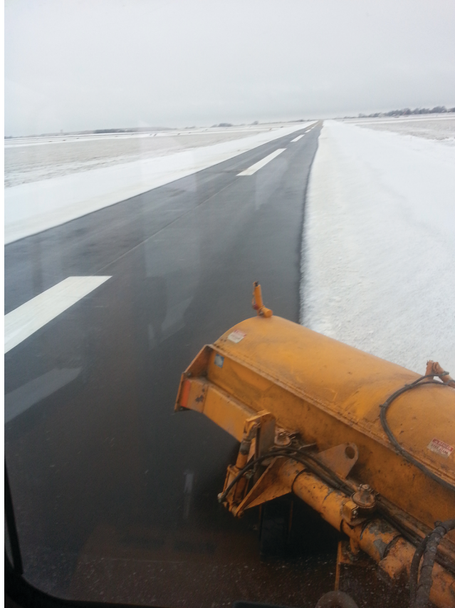
FIGURE 5 Example of pavement being cleared to a “no worse than wet” condition with a sweeper assembly. Photo credit: C. Lawson, Romeoville, Illinois.
