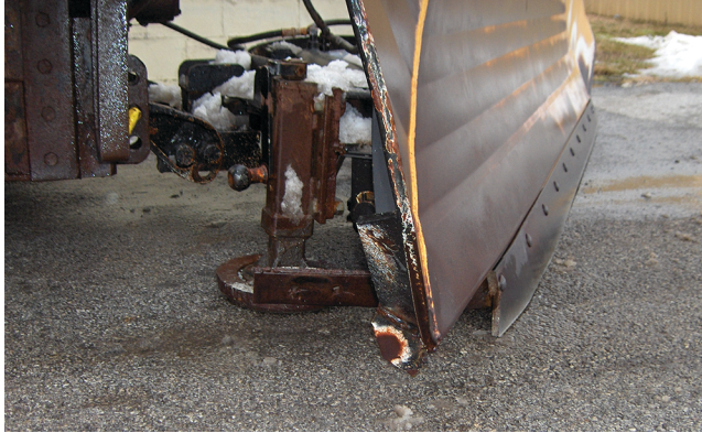
FIGURE 10 Example of plow damage not repaired due to budget issues. Photo credit: S. Quilty, SMQ Airport Services.
