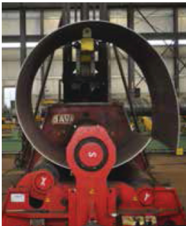
FIGURE 2 Rolling plate for pipe (left) and joining cans (right) (courtesy: Skyline Steel).
