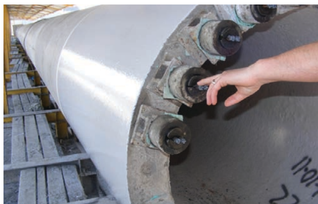
FIGURE 3 Spun-cast concrete cylinder piles; during casting (top; courtesy: Gulf Coast Prestress), after casting and still in forms (center) and during post-tensioning (bottom).
