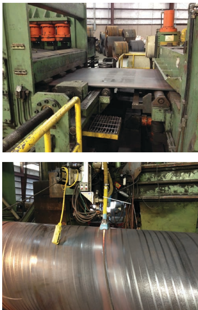
FIGURE 1 Spiralweld pipe: straightening the coil (top); note coils in background; and welding the seam (bottom) (courtesy: Skyline Steel).
