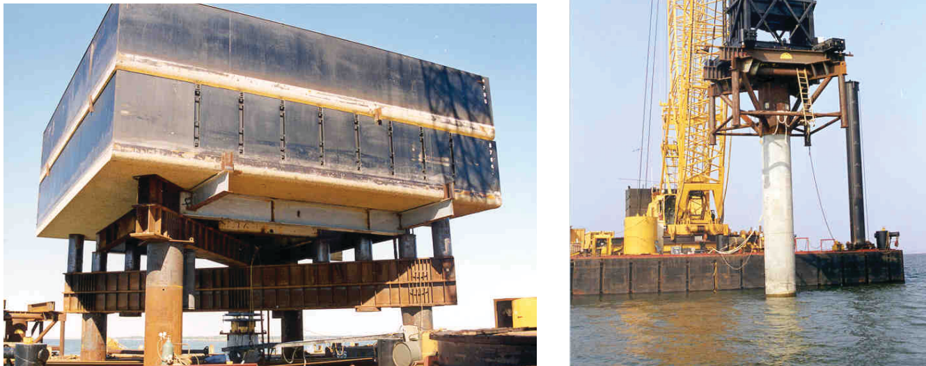
FIGURE 19 Static ( left ) and Statnamic® ( right ) load tests at St. George Island Bridge [Photos by Applied Foundation Testing (Copyright 2000)].
