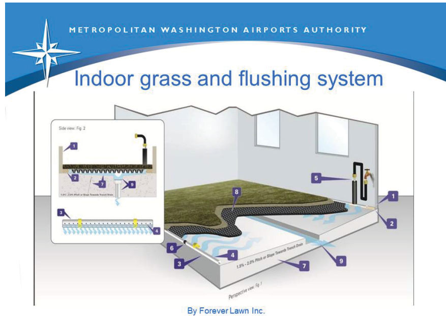
FIGURE 18 IAD's self-cleaning SARA Design (MWAA slide).
