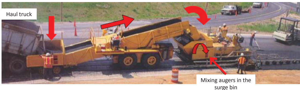
FIGURE 56 Example of a remixer in the surge bin in paver hopper [Source: Stroup-Gardiner (2014)].
