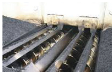
Pair of twin augers help pull mix from entire hopper and reblend mix as it is moved towards the screed.
