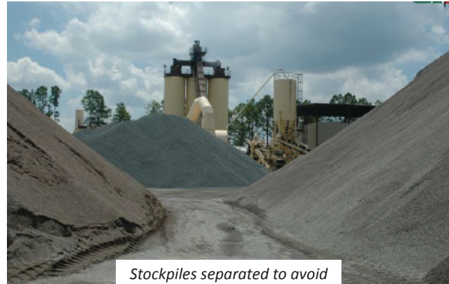
FIGURE 30 Course aggregates collect around the outside bottom edges of the stockpile [Source: Warren (2012)].
