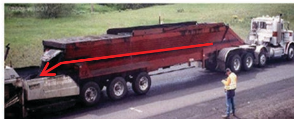
FIGURE 54 Live bottom haul trucks move mix horizontally and out the back of the truck bed [Sources: ABS Trailers ( http://www.abstrailers.com ) (upper left) and Pavementinteractive.org ( http://www.pavementinteractive.org ) (below)].
