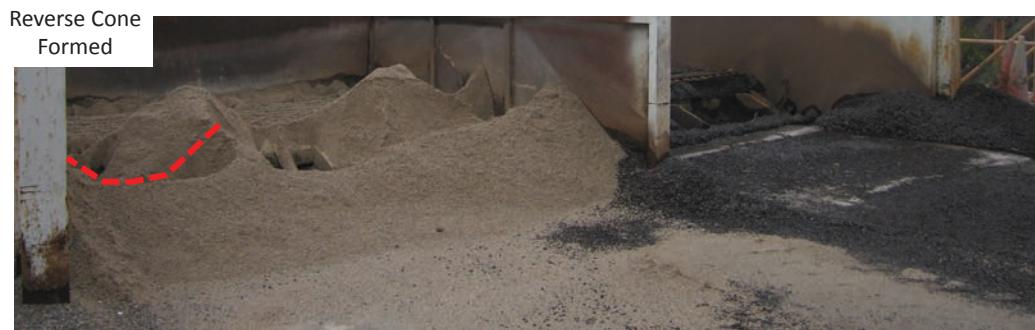
FIGURE 36 Reverse “cone” formed in center of cold feed bin which has been run too low [Source: Stroup-Gardiner (2014)].
