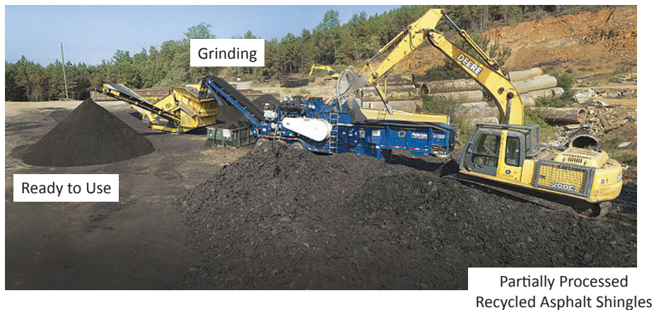
FIGURE 33 Several steps may be needed to process recycled material so a uniform, consistent size is obtained [Source: National Asphalt Pavement Association (n.d.)].
