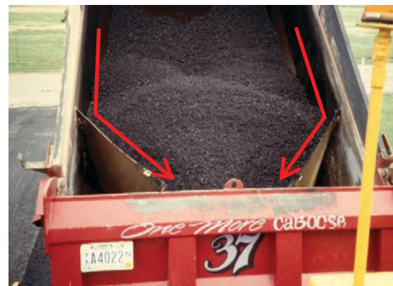
Baffles which create a funnel at the tailgate helps reblend mix as it exits.
