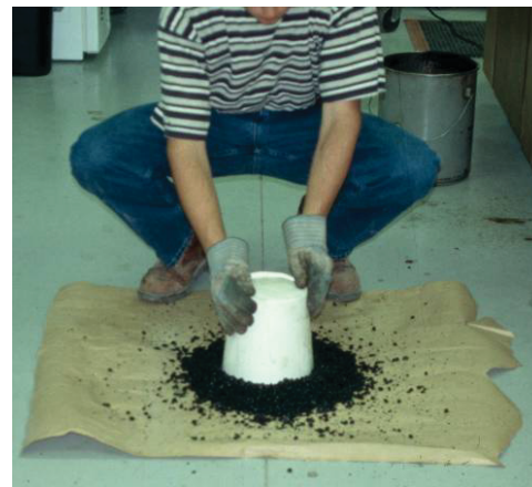
Material inside the bucket diameter is tested and compared to the results for the material outside of the bucket diameter
