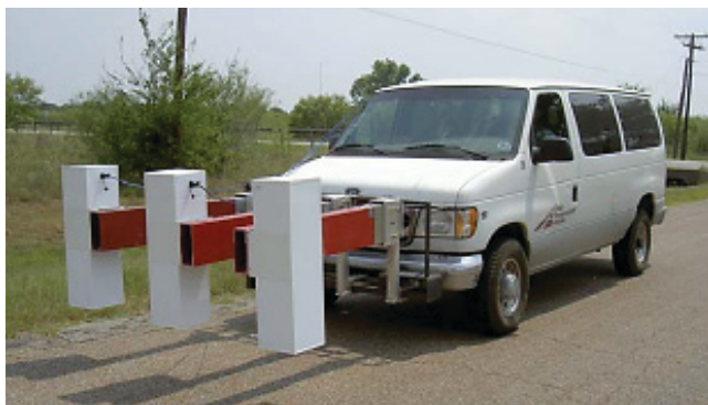
FIGURE 24 GPR vehicle developed by Texas Transportation Institute [Source: Sebesta et al. (2006)].
