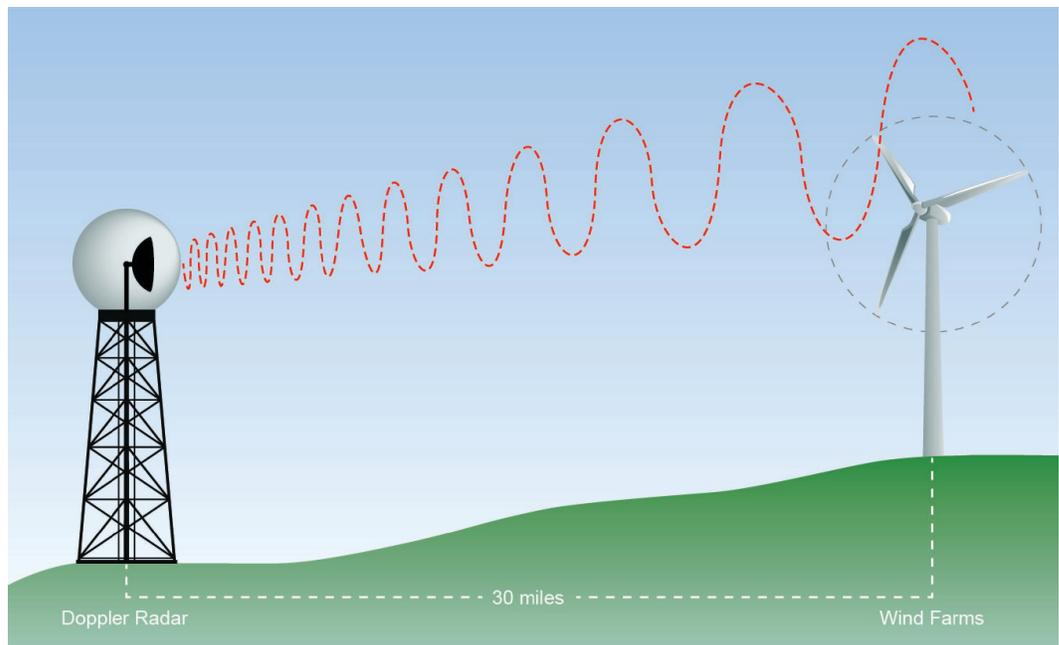
**Figure 2-18.** *Wind turbines as physical obstructions to radar signals.*
