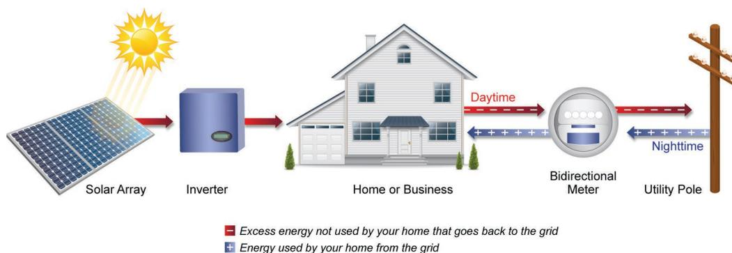
**Figure 2-10. How net metering works.**
