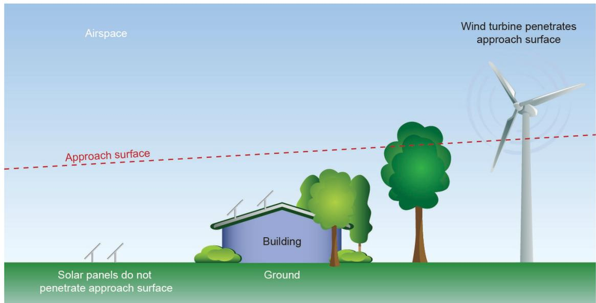
**Figure 2-16.** Examples of structures that may impinge on airspace.
