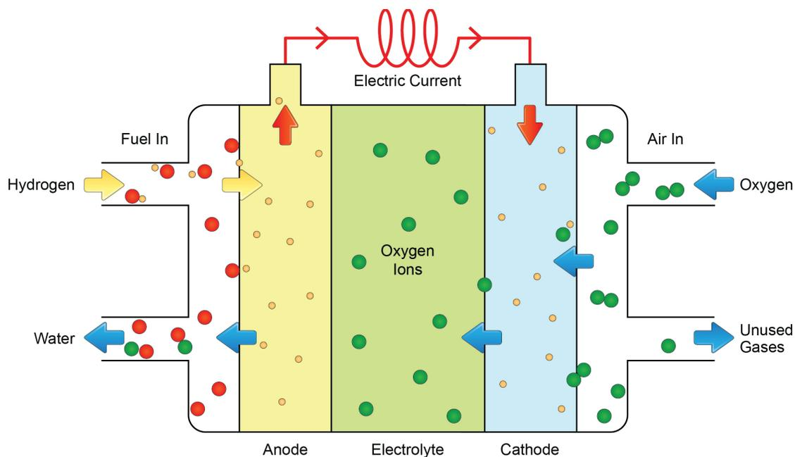
**Figure 1-16. Schematic of a fuel cell.**
