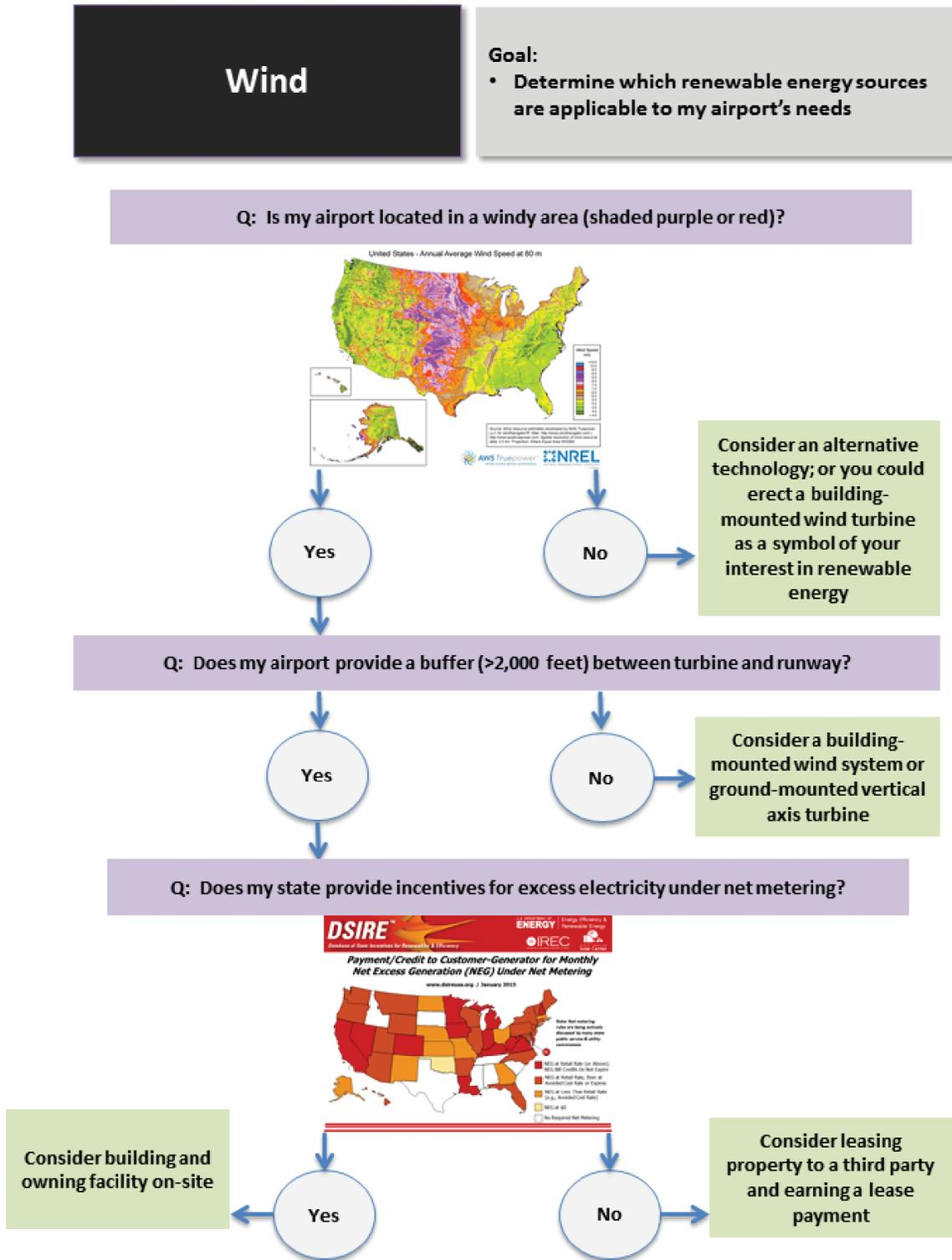
Figure 2-21. Wind process flow chart.
