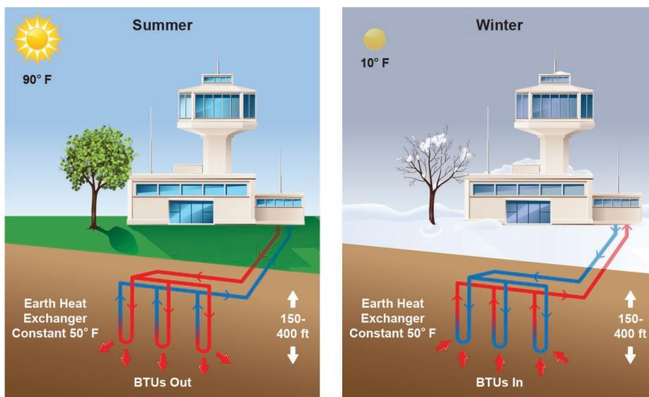
Figure 1-7. Schematic of geothermal heat pump.
