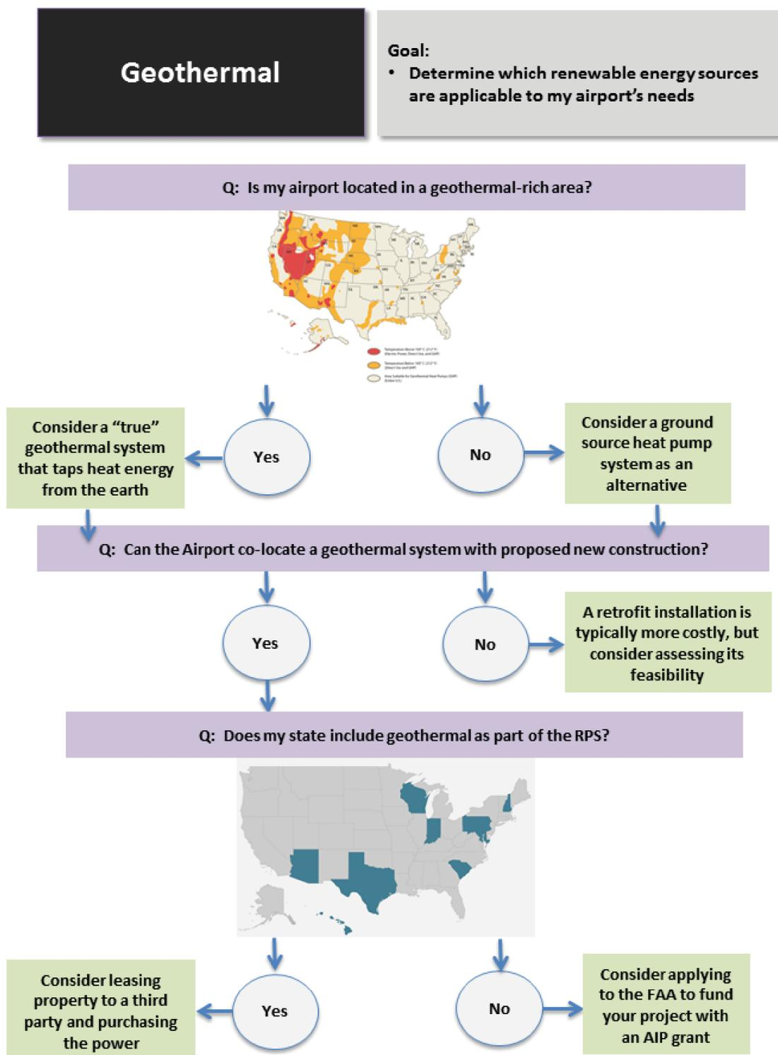
Figure 2-22. Geothermal process flow chart.
