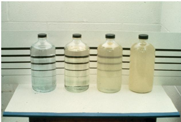
FIGURE 23 Different contamination levels of jet fuel. (Courtesy: Precision Filtration Products; used with permission.)
