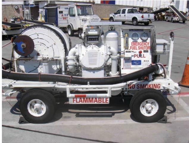
FIGURE 10 Example of a towable hydrant transfer cart. (Courtesy: S. Quilty, SMQ Airport Services.)
