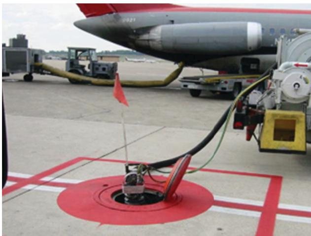
FIGURE 29 Marking and flag identification of fuel hydrant pit.
