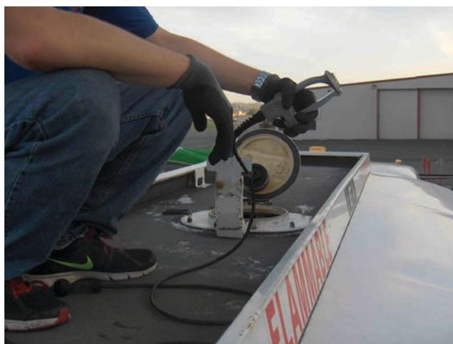
FIGURE 26 Example of employee monitoring mobile tank fill and operating an enabling switch. (Courtesy: S. Quilty, SMQ Airport Services.)
