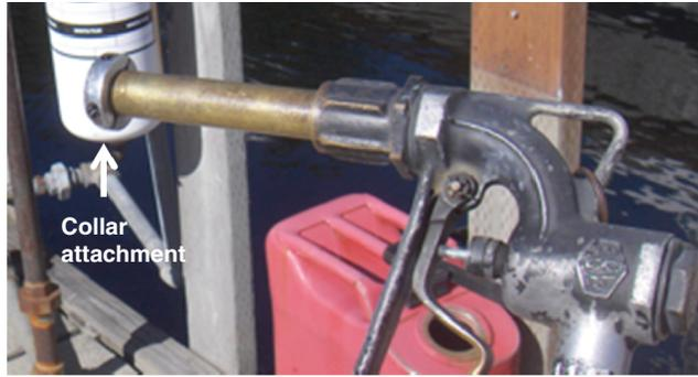
FIGURE 18 Collar attachment to nozzle to prevent fueling of jet fuel into avgas aircraft. (Courtesy: S. Quilty, SMQ Airport Services.)
