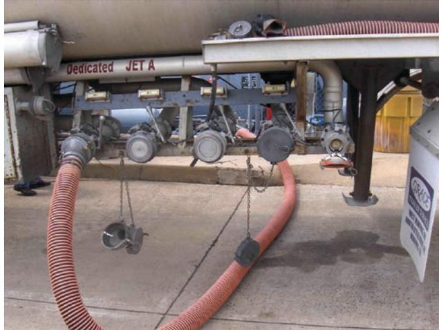
FIGURE 4 Example of a dedicated Jet A tanker delivering fuel to an airport tank farm. (Courtesy: S. Quilty, SMQ Airport Services.)
