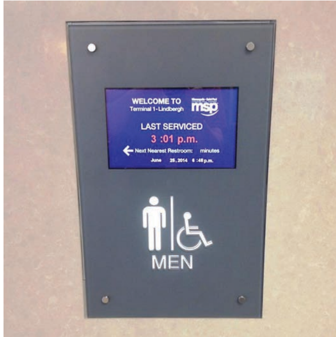
Figure 3-3. RMS with information monitor and backlit room sign. The card reader to activate maintenance features is located behind back-painted glass below the sign.
