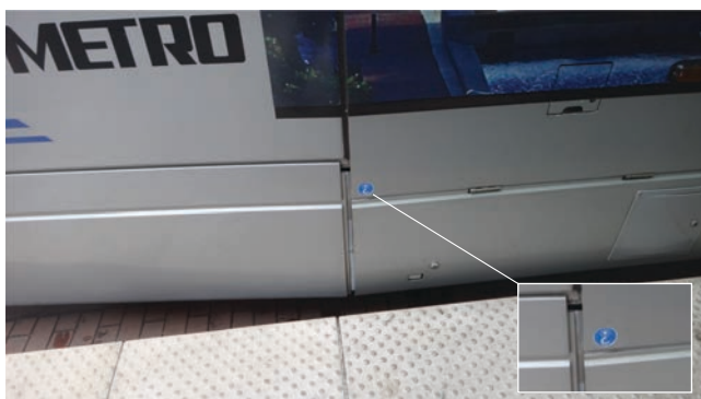
FIGURE 8 Example of lift point decals (center) on Houston METRO rail vehicles.
