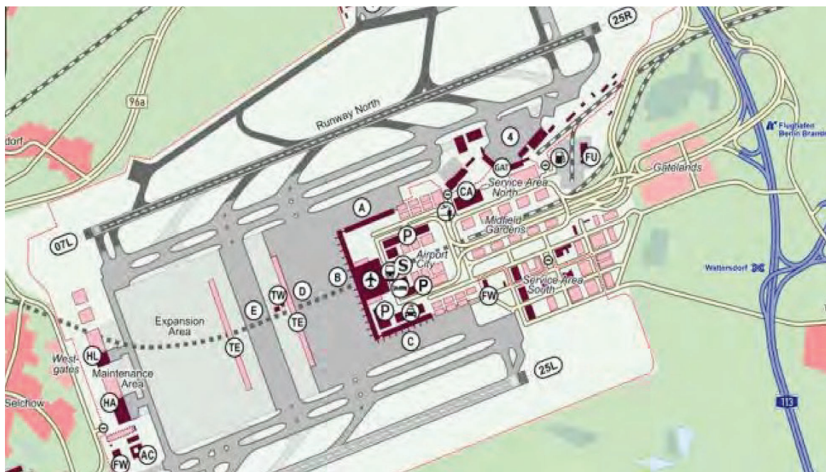
Figure 12-6. At Berlin Brandenburg Airport, the rail line is in a tunnel through the airport, allowing a through-routed rail station, shown by the symbol “S.” Source: Berlin Brandenburg Airport.
