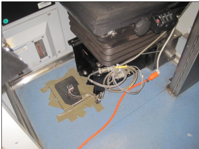
Figure 17. Carbody Accelerometer in Driver's Cab
