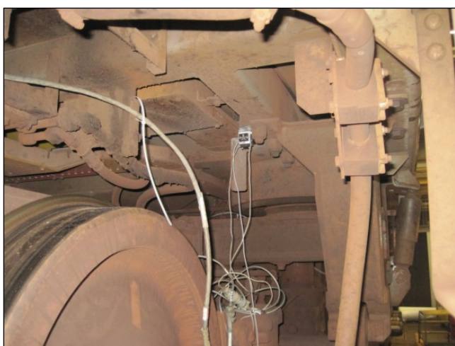
Figure 15. Carbody Accelerometer at Truck Centerline
