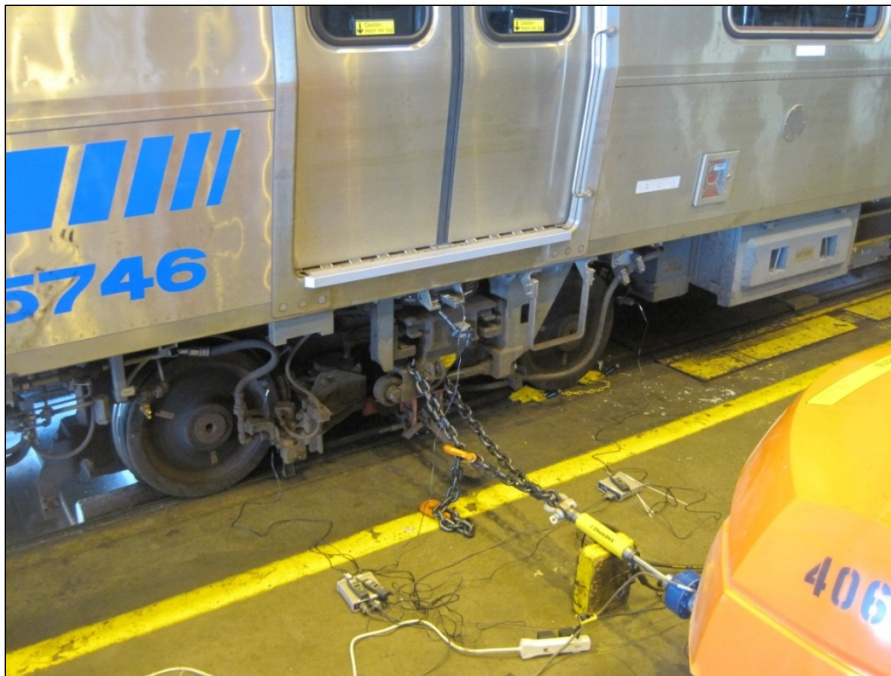
Figure 9. Lateral Stiffness Test Setup
