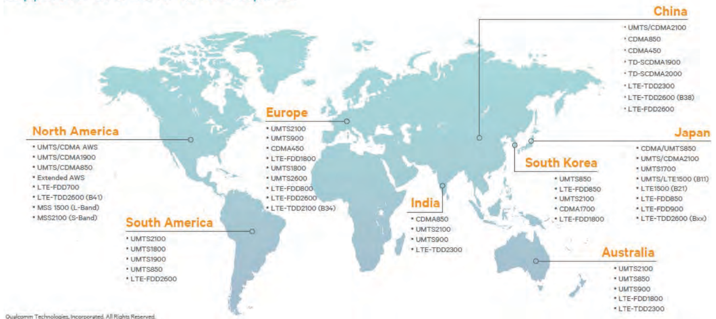
Figure C-2. A mobile device must support over 40 RF bands to be fully international. 32
