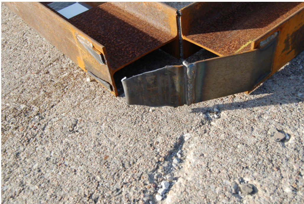
Figure 7: Bent plate post after test (TEST SDCB-2).
