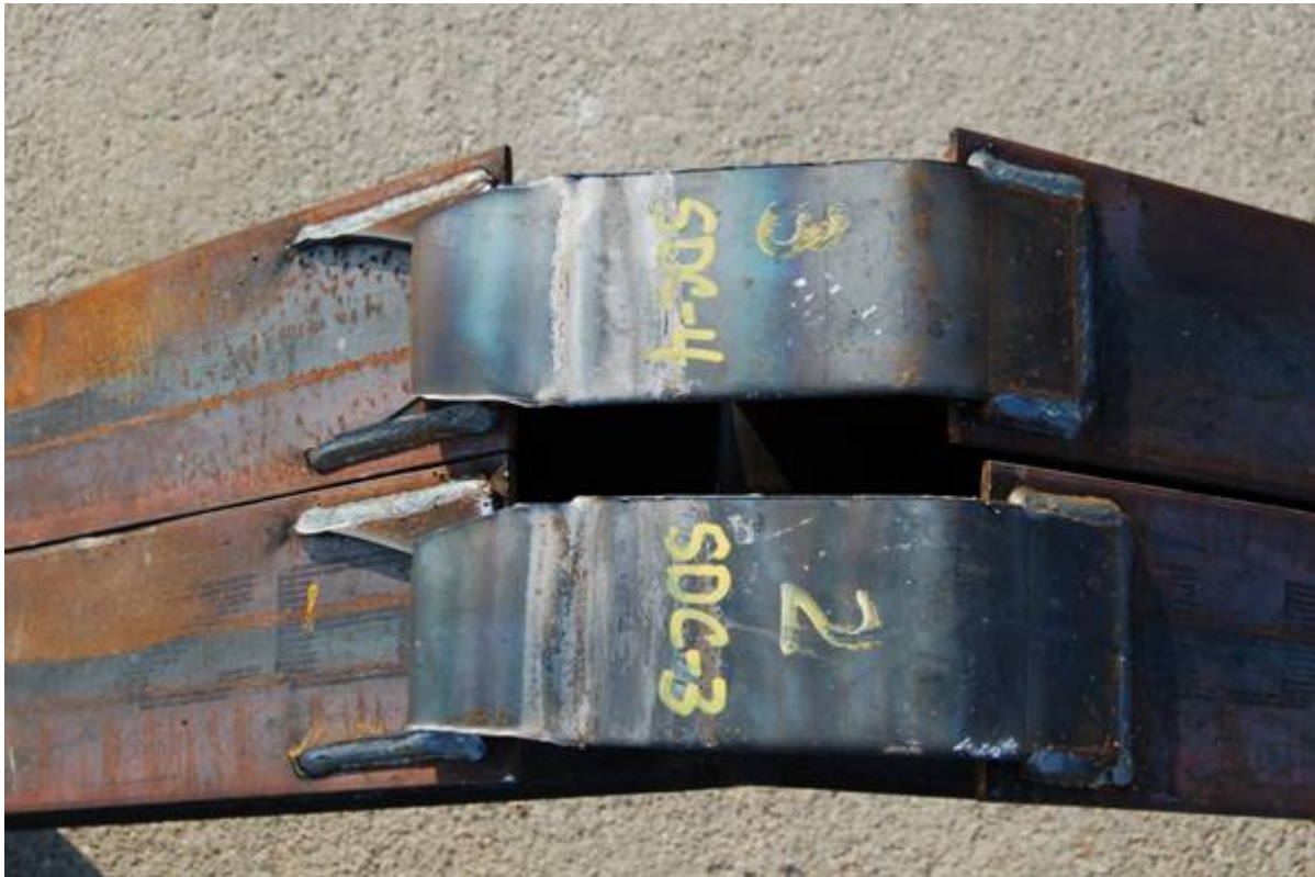
Figure 11: Photographs of posts after tests SDCB-3 and SDCB-4.
